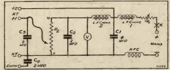
You will see that the circuit is fundamentally simple, the voltages being varied by R<sub>1</sub> and by the position of the flex clip from H.T. + 1. The point marked X near the + mains point is the alternative position for the H.F. choke, to suit some mains, as explained in the article.
