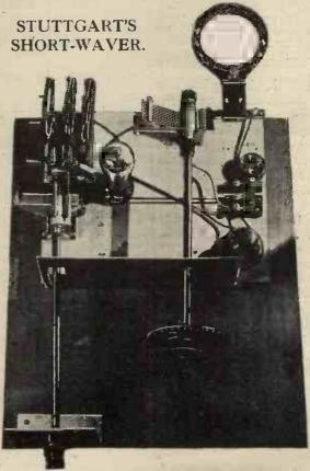
The simple short-wave receiver used by Stuttgart for picking up American broadcasts for relay purposes.
