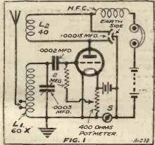
A highly-efficient one-valve circuit suitable for a small portable.
