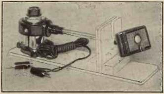
The "Blue Spot !! Pick-up is provided with a wooden "cradle" mounting to ensure safe travelling.
