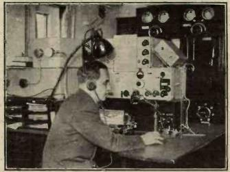
The received Morse messages are not written out, but are typed direct by the man wearing the 'phones. The operator on duty when this photograph was taken talking by telephone to the officer on the bridge as the vessel was preparing to leave Southampton on her record-breaking run.
