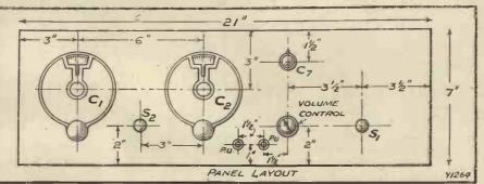
Here the position of the holes you have to drill in the ebonite panel are clearly shown.
