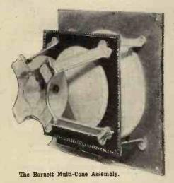
complete loud speaker of unusual design. The smallest cone, which is there presumably to handle the high notes, is arranged so that it is directional towards the back of the assembly. However, the arrangement does give good results, despite the abnormal mass locked to the driving spindle. With a unit of average price, the complete cost of the outfit is round about the £2 10s. mark, and bearing this in mind one has to admit that it is an unusually interesting proposition.
