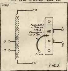
A two-pin plug-in "X" coil may be employed instead of a 6-pin aerial coil.
