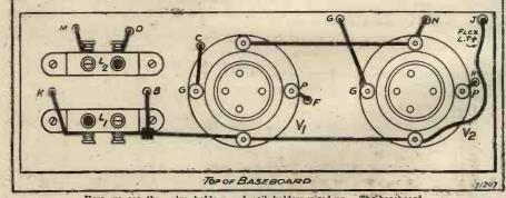
Here we see the valve holders and coil holders wired up. The baseboard fits above the panel and at right angles to it.
