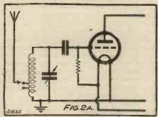
A tapped coil of the "X" variety increases the selectivity of a simple circuit.
