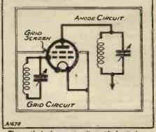
The method of screening the grid circuit from the S.G.'s anode circuit.
