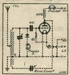
The dotted lines show the connections of the 1-valver given in last week's "Wirelet." It will be seen that a crystal and extra 'phone terminals are provided across the tuning condenser, so when the L.T. Battery is being charged the 'phones can be moved from 1 to the "Phones 2" position, and you then have a crystal set. To return to the valve instead, you simply replace the 'phones in the "'Phones 1" position.
