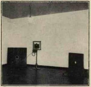
The smooth floor, bare walls and ceilings shown are specially arranged for loud-speaker tests, echo effects, etc., in this room of the Heinrich Hertz Institute, Berlin.
