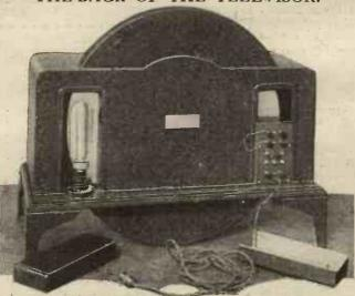
The rear of the televisor has two compartments, which, when the covers are removed disclose, (left), the neon lamp and, (right), the input motor voltage terminals.
