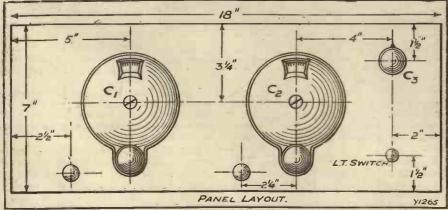
The panel preparation is well within the powers of the inexpert constructor, and, when he has done this, a big part of the work of assembly is completed.
