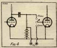
The leaky-grid detector requires a switch, two terminals and a G.B. lead. When the pick-up follows a transformer or a resistance stage (Figs. 3 and 4), it is a case of "fit and forget," as the same battery adjustments do for radio and gramophone.
