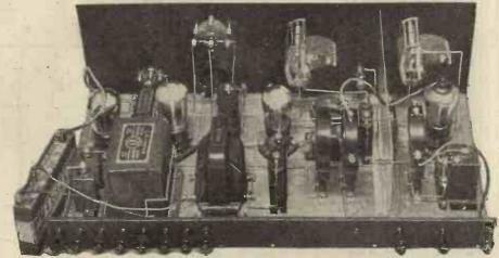
The layout of components arrived at makes the set delightfully easy to assemble, although an extraordinarily high degree of efficiency has been achieved. Note the very simple but most effective screening.
