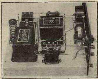
In the foreground is the  $C_n$  smoothing condenser, and immediately behind it is the potential divider  $R_o$ . The terminals on this are numbered as shown in the wiring diagram overleaf, and a fiex lead from the condenser is fixed to the required terminal before "putting the lid on." Simple isn't it? And SAFE 1
