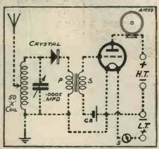
The dotted lines show the connections of the crystal and one valve amplifier given in last week's "Wirelet." (This class of receiver is very useful for obtaining loud-speaker results from a station situated only a few miles from the receiving aerial.)
