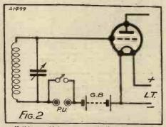
Nothing could be more simple than the case of the anode-bend detector
