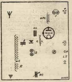
Here are the "components" for a straightforward one-valve set, using condenser-controlled reaction. It will be seen that a second pair of 'phone terminals and a crystal detector are included, the idea being that these can be joined across the tuning circuit so that the set will act as a crystal receiver when the battery is away "on charge."
