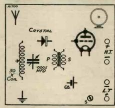
Here are the "components" for a crystal-and-one-valve set, as used for lond-speaker work near to a B.B.C. main (or very near to a relay)
