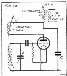
A typical circuit employing swinging-coil reaction.
