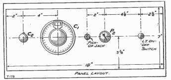
The panel is just like the "Magic" Three's, except for the pick-up tack and the volume control (P2).
