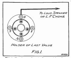
This is the wire you have to disconnect in order to insert the milliammeter when you use it to check the power valve's activities.
