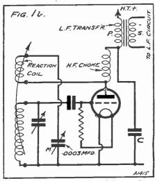
The circuit of Fig. 1a changed to capacitycontrolled reaction.
