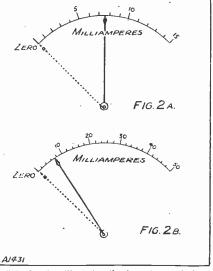
This drawing illustrates the importance of the relative sizes of the scales of meters. Notice the distances covered by each of the needles to indicate the same one or two milliamperes.
