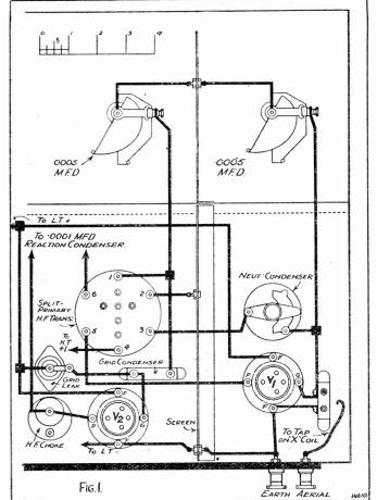
The H.F. side of a set employing a straightforward circuit, which can be modified quite easily to accommodate a screened-grid valve.
