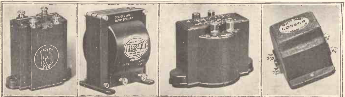
The R.I. "Hypermu" transformer (left) makes use of magnetic material of high permeability and is capable of giving a very excellent response curve. Next, we have the well-known Ferranti A.F.50. This instrument has a ratio of 3-1 and a primary inductance of 120/150 henries. The Igranic Type "J" transformer (third from left) weighs only 10 ozs. and is very suitable for sets where space is limited. On the extreme right is the Cossor transformer which has a ratio of 3-1 and a large primary winding.
