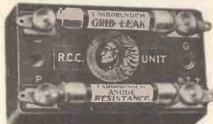
In the Carborundum Company's R.C. unit the anode and grid resistances are readily detachable.
