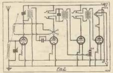
This "P.W." circuit necessitated seven variable controls, a D.P.D.T. switch and three jacks. Even so, the "Titan" Three, with its one dial tuning, would beat it hollow, although it has one valve less.
