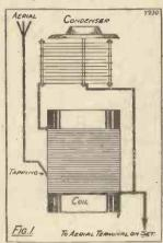
till it fades away (the jamming, not the condenser). The adjustment is pretty sharp, so the first time you try this arrangement you will have to move the condenser rather carefully.
