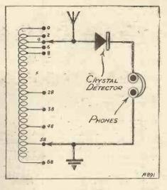
The ends of the flexible leads terminate with two spring tapping clips.
