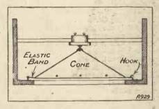
same from tearing, I got a bootmaker to insert in each a boot eyelet. Inside the speaker box are fixed eight small looks coinciding with position of the loles in edge of cone, which is suspended, as shown in sketch above, by eight small clastic bands. The bands being merely looped through the holes in the cone, it is a simple matter to renew them when they become perished.
