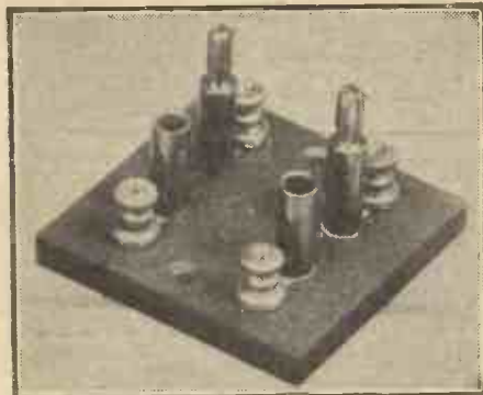
The two-coil holder. Single versions can be made up on the same lines, using a smaller base.
