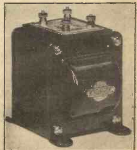
This component embodies the necessary items for one stage of dual-impedance coupling—viz., two L.F. chokes and a coupling condenser.
