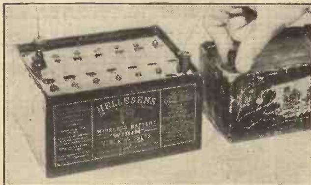
Never connect up a new H.T. battery in series with your old one, this being a very common cause of howling and poor results.
