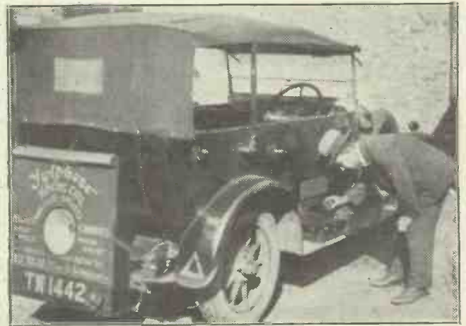
A demonstration car fitted up by an enterprising moving-coil loud-speaker manufacturer. The speaker is fixed on the back of the car. The operator is adjusting the gramophone and pick-up mounted on the running-board.
