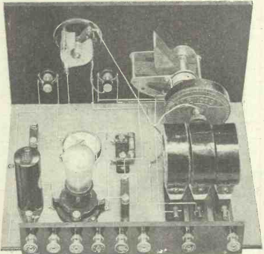
The low and high-wave coils were specially arranged to prevent objectionable inter-action effects, and the constructor should copy this part of the lay-out carefully.
