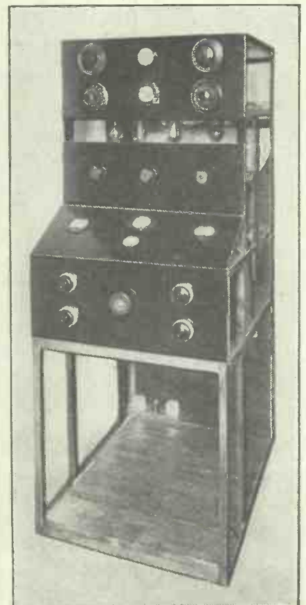
The completed transmitter stands five feet high, and is two feet wide.
