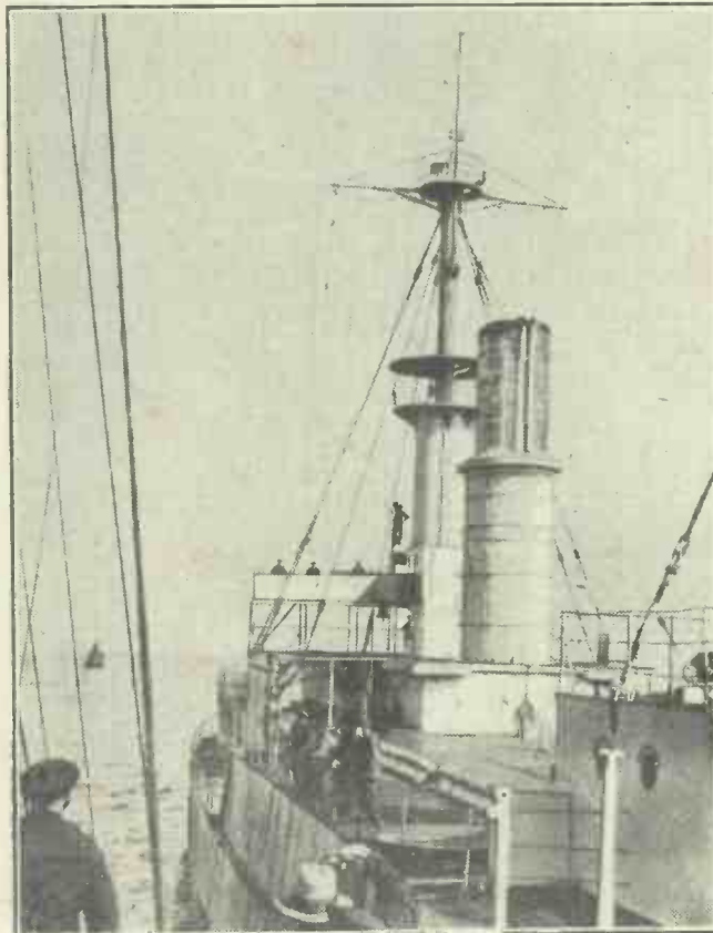
Here is the old German battleship "Zabringen," which has recently been re-conditioned for radio control. By means of wireless she can be steered and controlled at a distance without a soul on board her, and even if the control aerial is shot away another automatically rises in its place.
