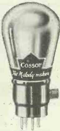
The Cosso five-electrode valve.
