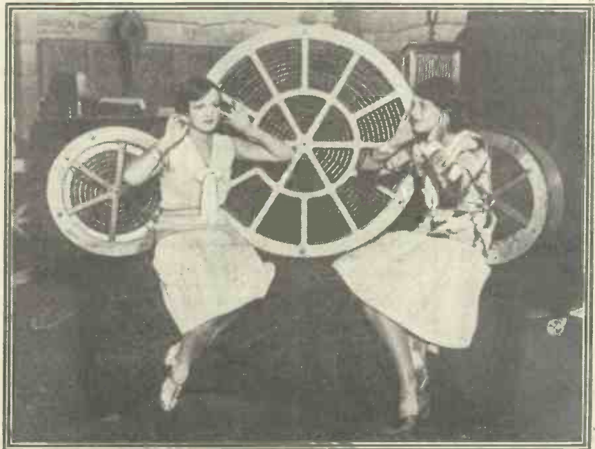
The loudest loud speaker at the National Radio Show at Los Angeles was this enormous one, with a voice that could be heard three miles distant. It is only intended for use in large halls, and consists of a thin diaphragm, three feet and a half in diameter, and resembles a cartwheel.
