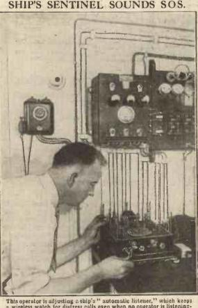
This operator is adjusting a ship's " automatic listener," which keeps a wireless watch for distress calls even when no operator is listening-im. All ordinary/calls are ignored by the selector device, but if an S O S comes along it rings bells in the operator's cabin, in the radio-room, and on the bridge.
