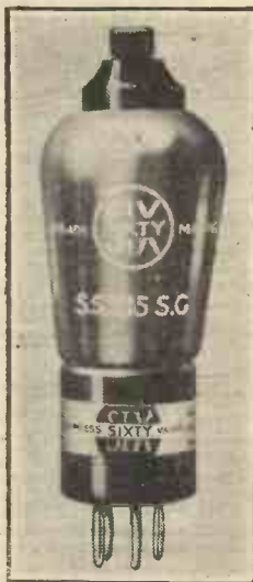
A Six-Sixty Screened-Grid Valve.
