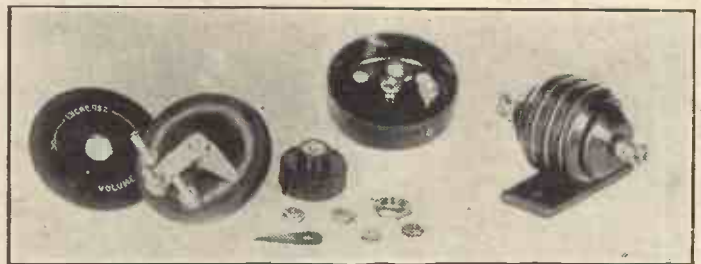
The high-resistance potentiometer disassembled and clearly showing the "pencil-line" along which the contact arm travels. The H.F. choke made by the same firm is shown on the right.
