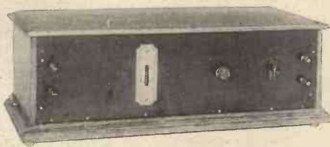
The filament switch on this set has a vertical movement and lends itself to clear panel marking in order to indicate its action.
