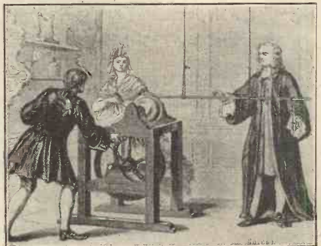
Fig. 2.—The discovery of the condenser. Imparting to a water condenser an electrical charge from a friction machine.
