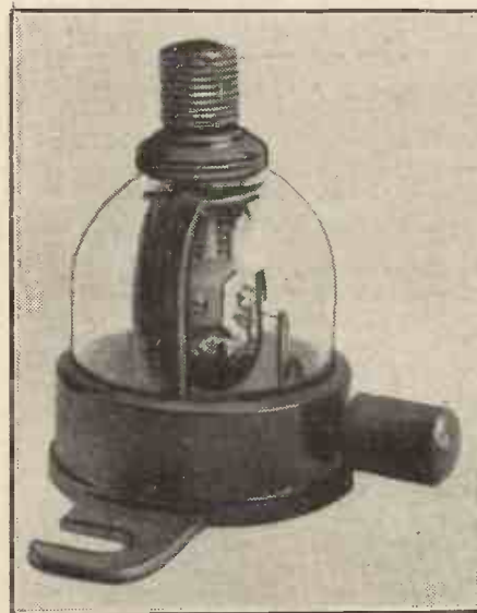
Fig. 4. A completely enclosed detector, in which the cat's-whisker contact is finely adjustable.
