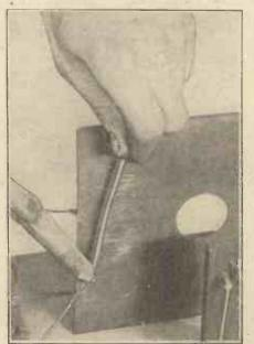
The solder should be placed in contact with the iron and the metals to be soldered, when a big joint is to be made.
