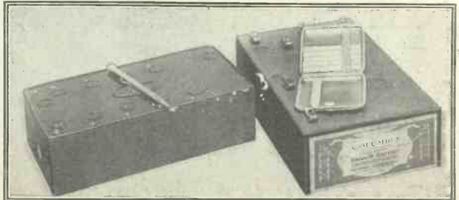
A sure way to spoil an H.T. battery is to short it. This can be easily done by carelessly putting a metal pencil, cigarette-case, or similar object on the battery. This is a sure way to spoil a battery that might with fair treatment have lasted months longer.
