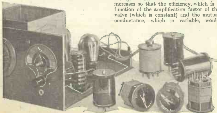
Some of the H.F. transformers which the author used in connection with the interesting experiments and tests described in the accompanying article.
