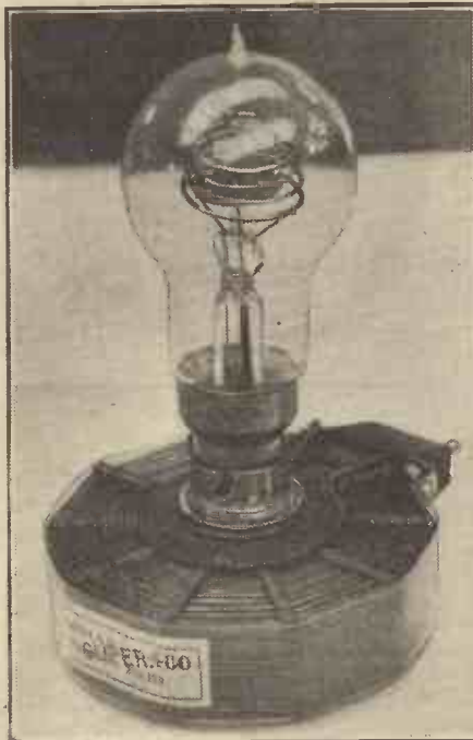
A novel test for a tuning coil is to make it light a Neon lamp by power picked up from a local oscillator.
