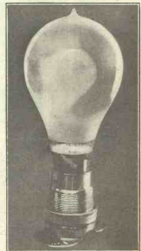
An untouched photograph of a 1911 electric lamp, which very clearly shows a "molecular shadow."
