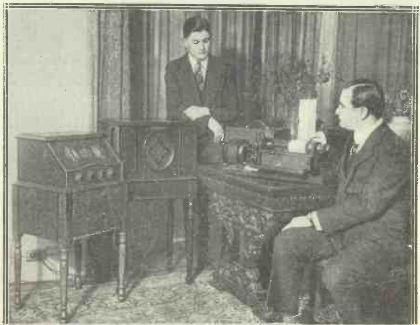
By means of the apparatus shown above, photographs sent from 111th Avenue, New York, via the Peumore (Long Island) broadcasting station, were picked up in the home of a New York scientist. After reception they required developing and fixing, just like an ordinary photograph.
