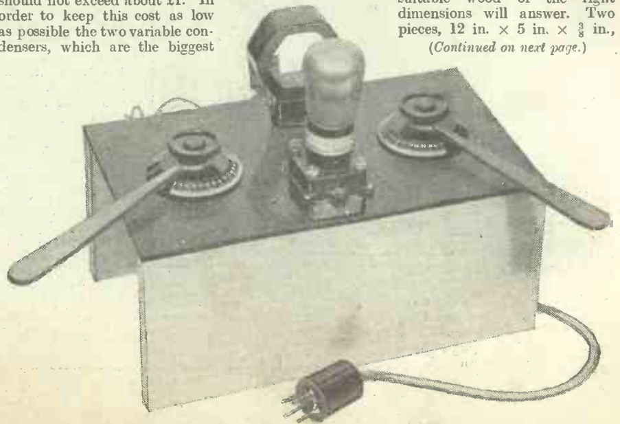
As shown, the panel is supported on two wooden sidepieces. Note the plug which goes into the detector valve's socket.
