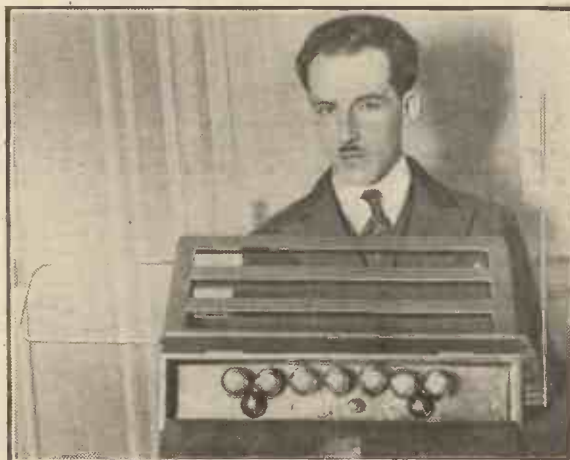
Prof. Theremin, whose "music from the air" recently created much amusement, some speculation, and a fair amount of controversy in this country, is now in New York, where he is busy endeavouring to mystify the Americans with his "magic box" (seen above). It is, of course, in essentials, an oscillating radio set, the "music" being controlled by a sort of hand-capacity effect.
