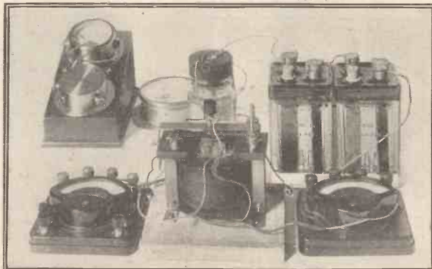
The complete universal charger "hooked-up" in an experimental form. Note the various meters employed for measuring input and output characteristics.
