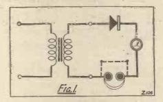
Fig. 1 shows a telephone transformer, to the secondary of which is connected a crystal detector in series with a sensitive microammeter. Now, if the primary winding is connected in the plate circuit of the detector valve, the rectified current
