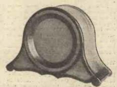
In some open-diaphragm loud speakers the back of the instrument is completely closed in.
