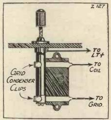
The fixed leak clips attached to the grid condenser have therefore become something of an unnecessary elaboration. but the method of fixing illustrated proves them still serviceable, one of them being used to make connection with the grid leak via the metal cap at the end.
