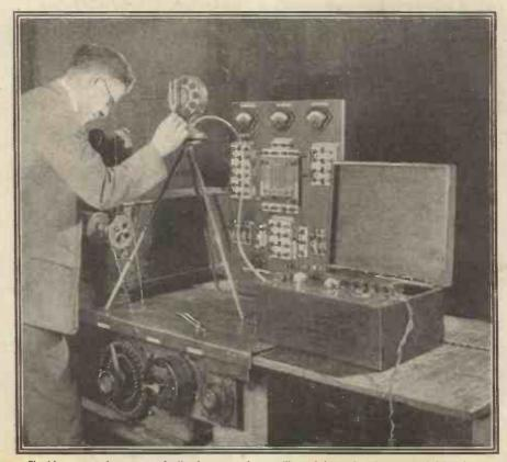
Checking up sound-wave reproduction by means of an oscillograph in an American research laboratory.
