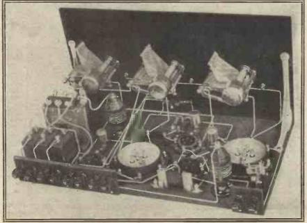
The lay-out of the "Logstation" Three allows ample wiring and component spacing without any sacrifice in compactness.
