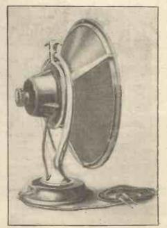
One of the earlier B.T.H. conical diaphragm speakers.
