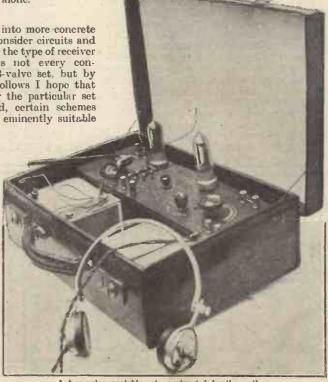
A two-valve portable set constructed by the author.
