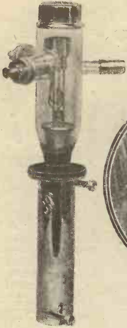
Above is shown, on the left, one of the modern high-power, water-cooled transmitting valves, and (right) the series of powerful generators and current converters used. The main power control switchboard is shown on the right.
