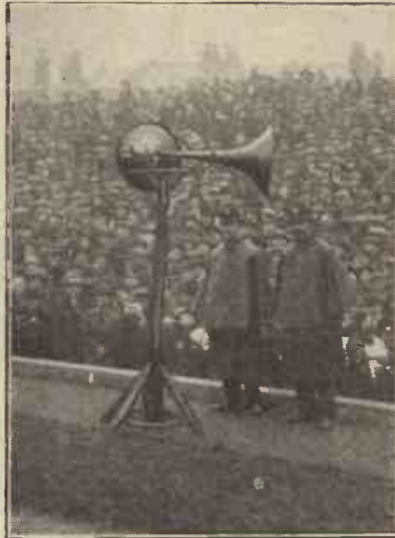
Large Amplion loud speakers used at the Highbury football ground in connection with the community singing movement.
