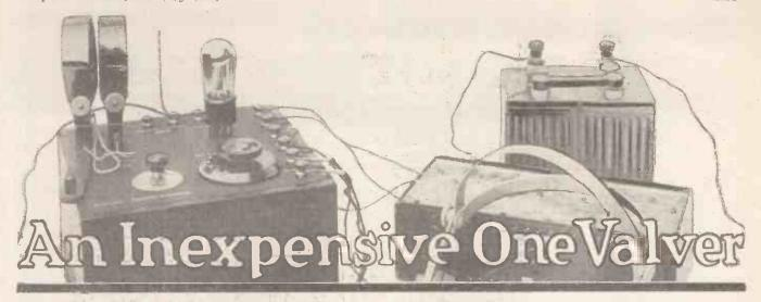
'HE outstanding features of this receiver are the ease with which it is made and operated, its reliability, and its low It is a straight one-valve set, with no "frills" of any kind, and if a homemade cabinet is used the total cost of the component parts should not be much more than 30s.
