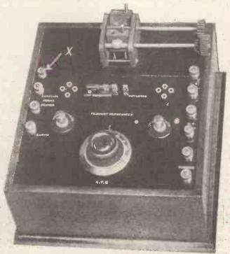
A straightforward set employing the popular "three-terminal" system with an extra terminal (marked X) corresponding with the additional terminal shown in Fig. 3.
