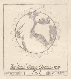
waves then combine to form a "stationary" wave system, the crests and hollows of which will be located in parallel circles extending outwards from the main transmitter.
