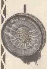
Back view of Coil showing arrangement of windings through the transparent cover. (Note the projection of the adjustment lever beyond the case, to obviate Hand Capacity effects.)
