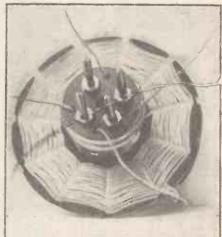
Fig. 3. Showing bow the leads are arranged.
