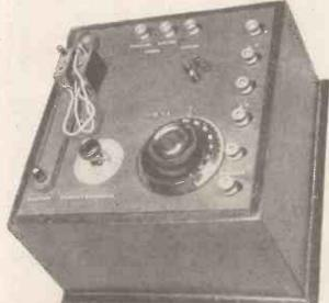
The coil holder and the tuning control—on the left and right respectively—are clearly shown in this illustration.
