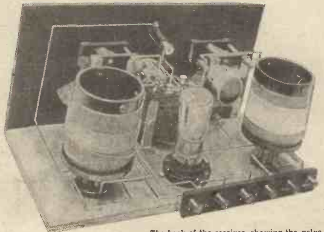
The back of the receiver, showing the valve and special H.F. transformers in position.
