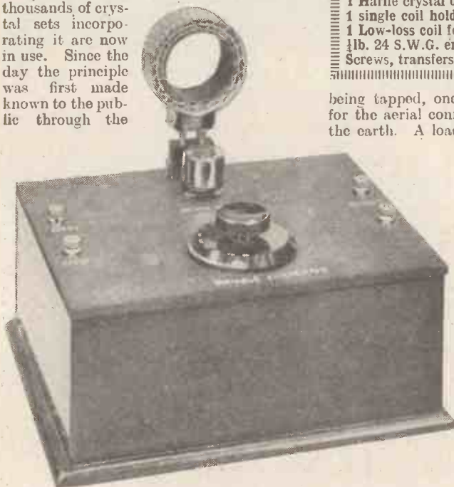
The completed set showing a loading coil in position of the panel lay-out.
