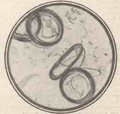
Fig. 6.—Microscopic coils of shellac as produced by the shellac insect.
