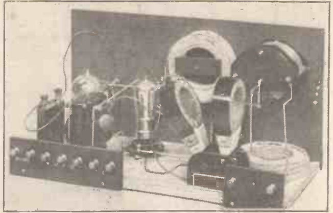
The complete set with grid bias battery, coils and valves in position.
