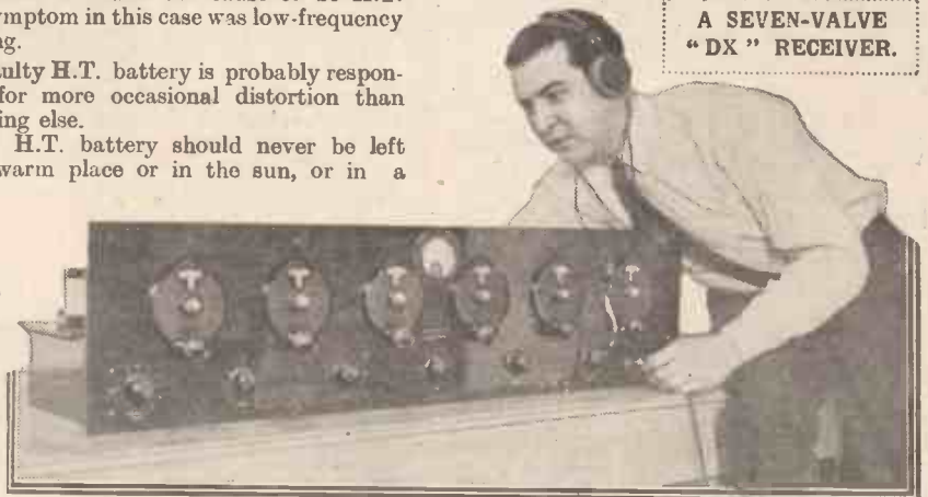
This American seven-valve receiver employs five stages of tuned high-frequency amplification, but is stated to be quite stable and easy to handle.
