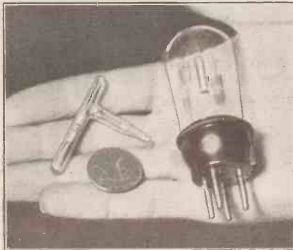
An interesting comparison. (Left) Mr. Marconi's first valve, made in 1895; and (right) one of the latest types of Marconi dull emitters. The coin is a halfpenny.
