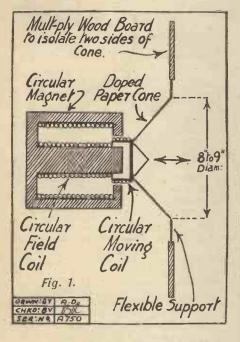
apex of a paper cone. The moving coil is situated in a strong magnetic field, and the currents in it react on the field. The coil, therefore, moves in and out in the directions shown by the arrows. The edge of the cone is lightly supported by some pliable material, such as stockinette or thin rubber, so that it can move freely.
