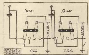
operate, is not complicated to wire, and has everything to recommend it. A type of switch similar in operation to this is the "Utility" which is very popular at the present time. A sketch of the "Utility" appears in Fig. 11, while the wiring of it is identical to that of the D.P.D.T. switch. A series-parallel switch of unique design is
