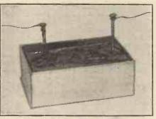
Fig. 3. A soot and sand grid leak.
