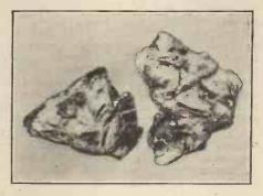
Molybdenite in appearance is of a leaden grey colour, without the minute crystalline structure which is so characteristic of galena. Usually it occurs in the form of flatlooking crystals. These masses of molybdenite are laminated, and, very often, layer after layer of the mineral can be peeled off very much in the same way as mica.
