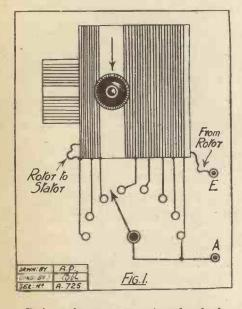
Perhaps the two most serious drawbacks to the variometer as an aerial tuner are the limited wave-length range obtainable, and the lack of selectivity.
