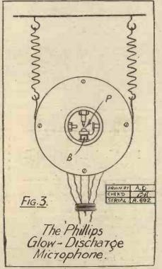
diaphragm vibrates and causes the pressure between the two buttons to vary. This alters the resistance of the whole circuit, so that corresponding current variations
