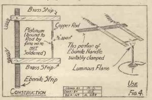
by varying the area of it which is immersed in the distilled water. Also, by adding minute amounts of common salt to the distilled water in the bottle, the resistance of the leak may be controlably lowered. (Continued on next page.)
