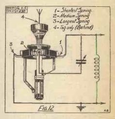
For placing the condenser in "parallel" with the aerial coil, the aerial lead is removed from the centre terminal and joined instead to the top terminal marked "parallel." The centre terminal at the same time is joined to the "earth" terminal. The condenser is now in parallel.
