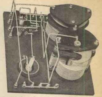
An under-panel view of the set which clearly shows the wiring to the battery terminals and secondary condenser.
