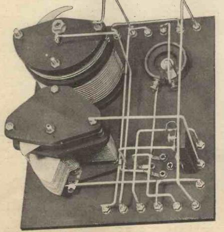
No difficulty should be experienced in wiring up the selective one-valve set if this illustration is taken as a guide to the connections.
