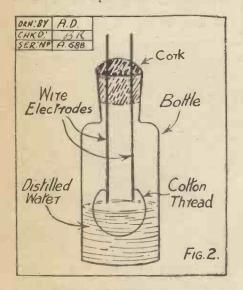
A grid leak, however, is not a difficult thing to make. On the contrary, it is probably one of the simplest radio components which it is possible for the amateur to construct. For the advanced experimenter, even, the subject of the grid leak is by no means final. It is quite possible that more efficient grid leaks may be devised, and that they may supersede the highly
