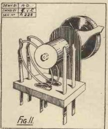
As the reader will observe, three terminals, about 1 in. apart, are utilised. One is marked "parallel," one "series," and the other "earth."
