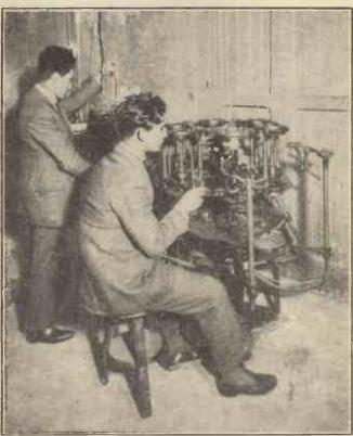
Some of the up-to-date valve exhausting apparatus installed in one of the Italian Radio colleges.
