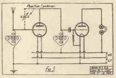
Moreover, since practically the whole of the tuning capacity is that of the aerial, the latter will have a very great influence upon the wave-length to which the circuit may be tuned by the variometer. Consequently it is difficult to predict the value of a suitable loading coil within close limits, and the correct size of coil should be found by experiment.
