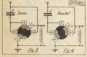
the condenser "all-in" will be approximately 30 to 50 metres below the actual wavelength of the coil (on the broadcast band of wave-lengths). As the condenser is rotated towards minimum capacity the wave-length is decreased. The drop in wave-length with the condenser in series
