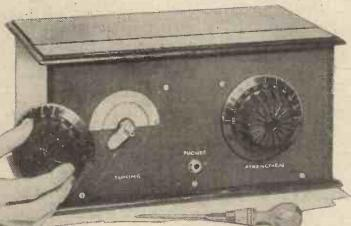
There are only three items on the panel: a 'phone plug and two dials. One of the latter is removed in the above photograph to show the wave-band change system.
