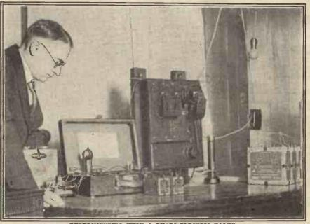
EXPERIMENTING WITH A PHOTO-ELECTRIC VALVE. An American physicist engaged in research with the new "Shadow-tube," which works like a valve, but is controlled by any shadow falling upon it.
