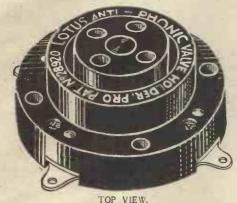
Valve sockets and springs are locked together by a mechanical process, making a definite and permanent connection. Bakelite mouldings, nickel silver springs and phosphor bronze valve sockets. Nickel plated.
