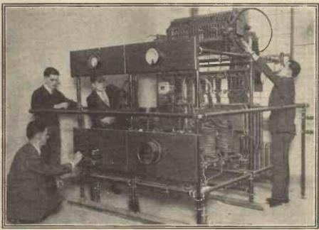
One of the transmitting panels at W J Z, which can now handle the super-power of 50 kilowatts.
