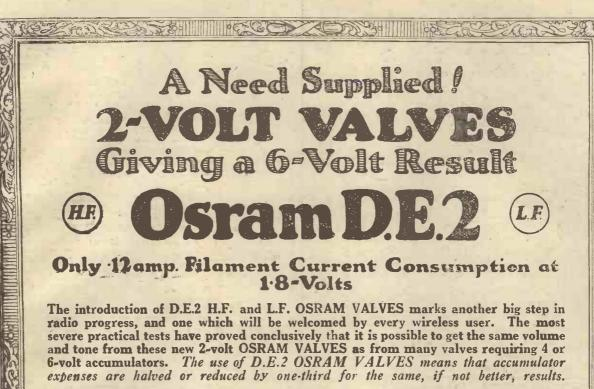
D.E.2 H.F. and L.F. OSRAM VALVES are developments from the well-known and popular D.E.R. class, but possessing better characteristics, a third of the current consumption and the same immunity from possible destruction by overrunning. You cannot over-run the D.E.2 with a 2-volt accumulator and a standard 5 ohms filament resistance.
