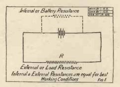
as follows: If a source of direct or alternating current *having internal resistance* is connected to a work or load circuit, then the maximum power is expended in the load (i.e. one gets the most useful working conditions) when the latter power is equal to the power consumed in the source itself.
