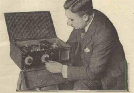
This completely self-contained American portable set is extraordinarily compact, as readers will agree when it's stated that an eight valve super-het circuit is employed.
