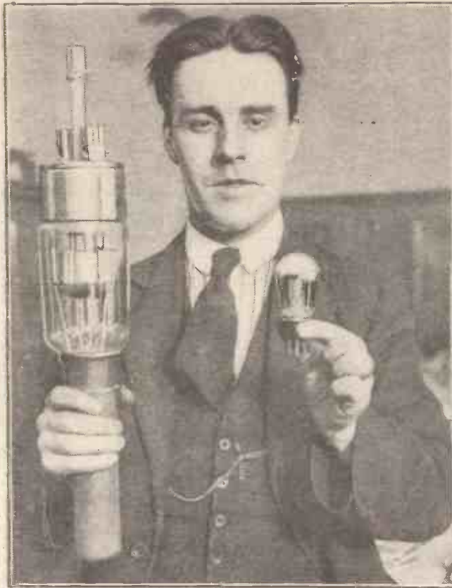
One of the new 10 kw. water-cooled valves in use at the Rugby Station compared with the average valve used for reception.
