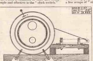
Showing Method of Mounting Clock & Switch.
