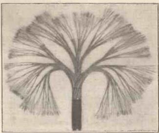
This photograph shows how the 6,561 strands of wire are twisted into one cable.
