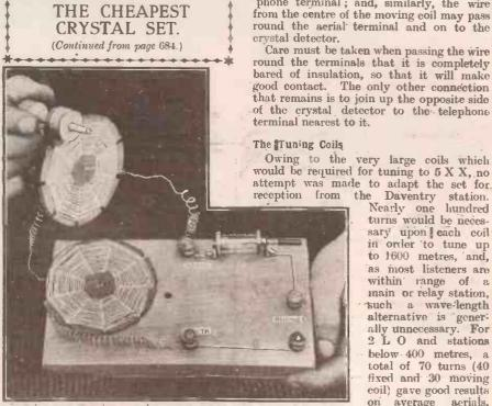
This photograph shows the moving coil connected up ready for placing in position on the panel.
