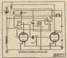
"P.W." Continental set in many respects. Also that the same varve will do the detecting in both circuits. A set like this should be popular with all as the two circuits are very much used. I have enclosed a small photo of myself with some sets I have made. The two-valve set is the same as your "Continental" set, except that I have placed the coils on the ontside of the panel.
