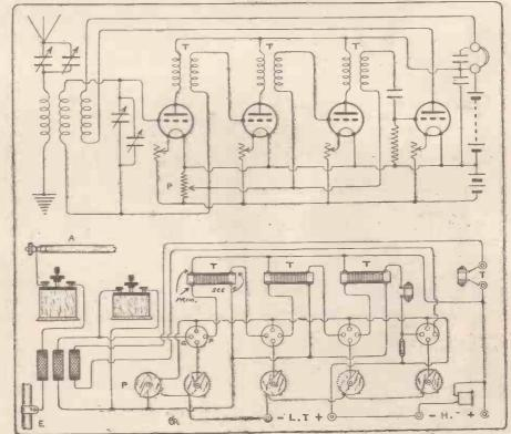
Fig. 8.—These diagrams show in theoretical and pictorial form an efficient four-valve circuit employing aperiodic transformers.
