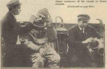
The diver being equipped with a microphone during some recent undersea broadcasting experiments carried out near Heligoland.
