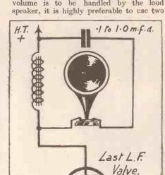
or more instruments in series or parallel, the use of a single loud speaker involving risk of overloading, which is the cause of a great deal of distortion in this stage.
