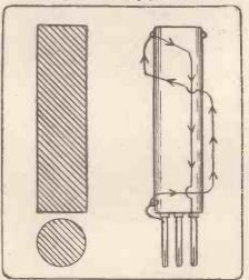
Fig. 2.—A plug-in transformer.
