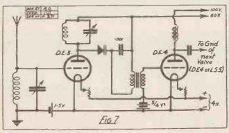
through a grid bias battery to an L.T. negative. The value of this leak seems to be of more importance when dealing with large input voltages, and it should then be about '25 to '5 megohms.
