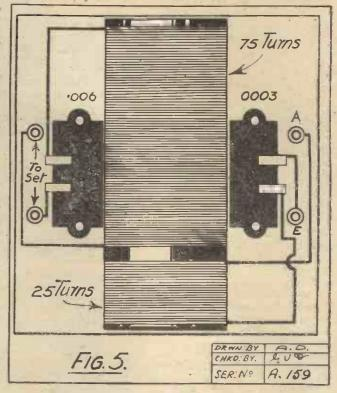
receiver. Where a 35 or 50 turn coil has been in use a 75 may be necessary. When series aerial tuning is used, the same law applies but at a slightly less degree, and a 100 turn coil may be required.
