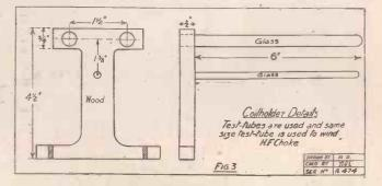
sliding them over the two test tubes and the glass rods of the coil holder, and to give a larger area of contact for the clips the coil ends should be slightly flattened by hammering on an anvil.
