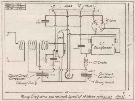
A study of the various photographs of the receiver will give a good idea of the relative. positions of the various components, and it. will be seen that no panel has been used, Instead all the components are mounted on a wooden baseboard 12 in. by 16 in. covered with American cloth.
