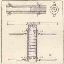
Fig. 1.—Constructional details of one type of transformer.
