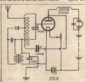
Here reaction is controlled by the small variable condenser C2, and with the correct number of turns in series, wound on the earth end of the coil, a smooth and easily adjustable form of reaction is obtained. number of turns for each tapping is the same as given above for No. 3, while 15 turns should be added for the reaction winding, which with a 0002 mfd. condenser in series, will cover the same wave-length bands. Below 300 metres it is more convenient to use 20 turns for the reaction
