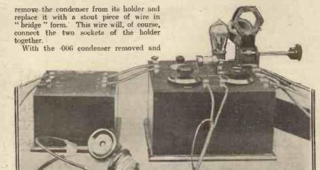
The "Automatic" Wave-trap connected to an ordinary one-valve and crystal-reflex receiver.
