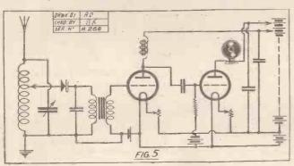
The rectified currents from the detector cause voltage fluctuations to be impressed upon the grid of the first L.F. valve, and these variations in grid voltage cause proportionate fluctuations in the anode current, which in amplitude and wave form are amplified replicas of the original rectified currents, but this is true only up to a certain point. The ratio of anode current change to grid volt change must be constant for distortionless amplification.
