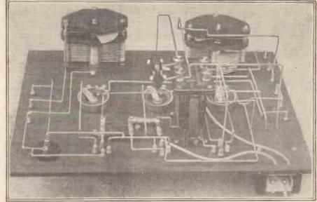
An under-panel view of the Straight 3-Valver showing the disposition of components and method of wiring.
