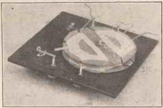
The method of "stopping" the rotating coil can be seen above, which shows the set before completion of the wiring.
