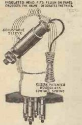
CLIMAX ANTI-MICROPHONIC VALVE SOCKET is made on an entirely new principle. The valve floats on metal springs. Each separate socket contains a patented hour-glass contact spring which is truly anti-microphonic and at the same time makes excellent electrical contact.
