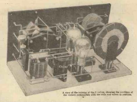
be avoided. Square section tinned copper wire is advised as it not only makes the set much neater in appearance but is easy to handle and an efficient conductor.
