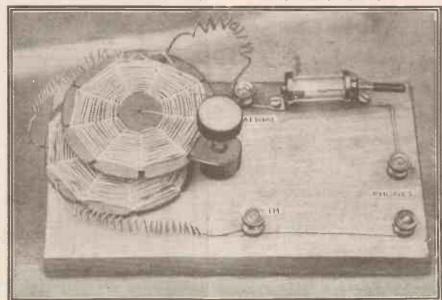
The complete set. Note how the cardboard former of the upper coil is fitted on the wooden disc through which the control-rod passes.
