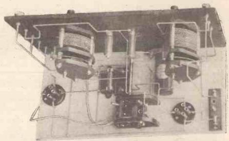
A photograph of the interior of the receiver taken after the completion of the wiring. Note the position of the H.F. choke.
