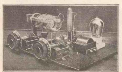
A three-quarter view of the 10-metre set. The transformer shown is of C.A.V. manufacture, while the valve holder is of American make.
