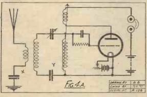
"tuner" should be connected to the aerial and earth terminals of the receiver to which the instrument is to be attached, aerial and earth leads being taken directly to the terminals so marked on the "automatic."
