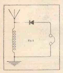
accurately determined, the tuning coils can be wound so that the tuning of the whole system will respond to the exact frequency of the waves from the station from which it is desired to receive, without further refinements such as variable inductances or tuning condensers, but up to the present time the cost of the instruments required for making the necessary measurements has been altogether out of proportion with the saving effected in dispensing with tuning devices.
