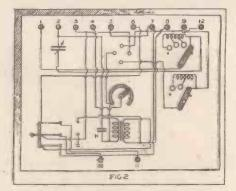
circuit, which is used for obtaining low-frequency amplification. When on the valve side this transformer serves to feed the low-frequency currents of the crystal circuits into the grid circuit of the valve.
