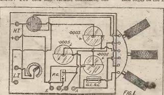
0003 mfd. variable condenser, three-coil holder, basket or honeycomb coils, rheostat, grid leak and condenser, 001 fixed condenser, valve holder, eight terminals.
