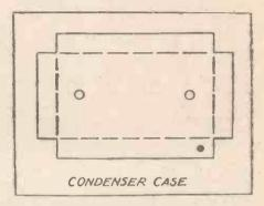
record till it is easy to bend, then bend as shown by dotted lines, bringing the corners together. The corners may then be rounded off and sealed with a hot iron, such as a poker or anything of that description. The case can then be finished off with glass-paper to the maker's satisfaction. This type of case has been thoroughly tested and has been subjected to 2,000 volts A.C. between holes and through the thickness successfully, no sign of leakage being noticed.
