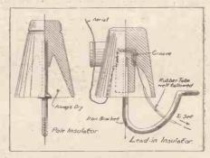
egg, rec!, or barrel insulator. Having found these quite useless in preventing leakage by wet, I tried the ordinary house telephone insulator, and I have found a marked inprovement in reception. Another item is the lead-in tube, the usual conventional type, ebonite tube with brass rod and nuts, being quite unsuitable in wet weather. The above insulators answer admirably. They may cost a little more, but they make up for that by solving a problem. The above diagrams show my arrangement.
