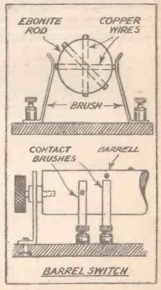
hammered over to make a rivet and good contact. It will be evident that after a turn of 180° of the barrel the pair first in contact will be again in contact. The several pieces of copper wire passed through the barrel must, therefore, be included within a range of 180°; say, at angles of 30° to one another. A dial may also be added, so marked as to indicate which of the contacts is being engaged.
