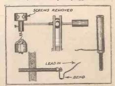
the other. Should it be impossible to split the pin, the same effect is obtained by flattening the thread slightly until it fits tightly.
