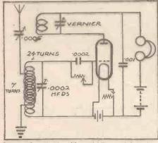
A one-valve circuit with a tightly coupled aerial and closed circuit with which short wave American stations have been clearly received in this country.
