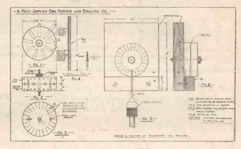
upon this. The simple "gadget" illustrated in Figs. 5 and 6 will, however, remove the main difficulty and enable the veriest novice to do this successfully.
