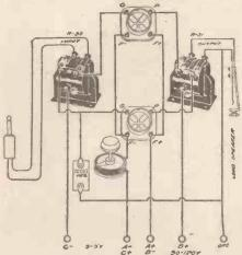
A "Push-pull" amplifying circuit using the special transformers mentioned below.
