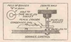
rubber sheet, such as a circular eraser. From this latter cut out a circular piece about half an inch in diameter, and through the centre of this pierce a hole just large enough to enable it to be fitted tightly upon the valve-socket.
