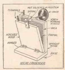
stationary piece and the other similarly on the movable piece, these being connected respectively with the two sheets of tinfoil, which are the "plates" of the condenser. The distance between the plates is regulated by means of a screw operated by a knob, as shown. Other methods of adjusting the distance may, however, be adopted as may be convenient.
