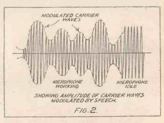
the wire; this effect can be detected by a wireless receiver. The more frequently the electrons—or the current—change direction and swing to and fro, the farther off is this peculiar effect noticeable. In brief, when the current oscillates extremely rapidly, it causes ripples or waves in the ether which (Continued on page 570.)
