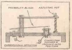
black composition found inside the coil, slightly warming first. By screwing two battens to the underside of the base, the whole detector is then complete. A glance at the diagram will explain;
