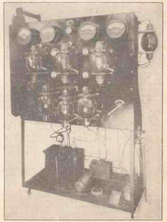
The modulating and oscillating panel at La Presse, the Montreal broadcasting station. The huge 2,000 watt valves were made in England.
