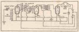
The three-valve circuit with which Mr. Rogers heard K D K A last winter without using an aerial. The last valve was ultimately cut out.
