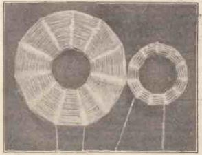
Showing the anti-capacity coils in their completed form.
