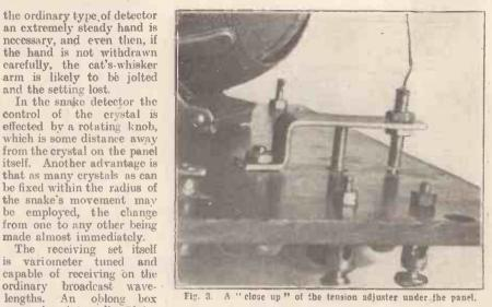
Fig. 3. A "close up" of the tension adjuster under the panel,
