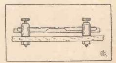
The terminals should be clamped to the ebonite about 2 inches apart, one being connected to the aerial and the other to the earth terminal in the usual way. The pen nibs are adjusted until there is a space of about  $\frac{1}{16}$  in. between their points, the small clamping screws then being screwed down very firmly.
