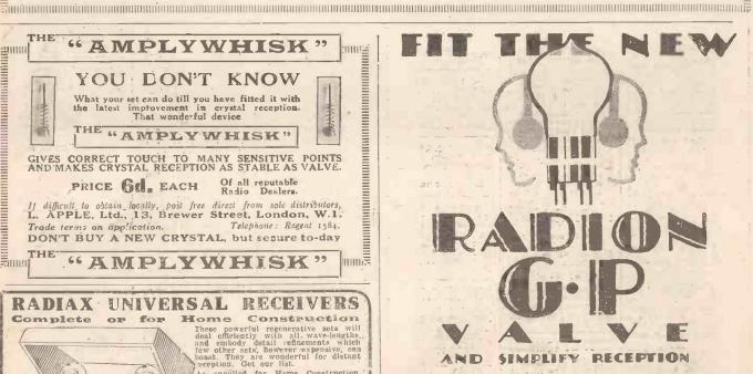
Here's an economical bright emitter general purpose valve with amplification factor of 9. Filament 3.5 to 4 volt '48 amp.' Anode 30 to 90. Use it in any part of your set. Let us send you free and post free the curve for this valve. Just a P.C. will do.
