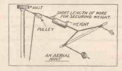
drawing down the part of the rope which was attached to the aerial, so that you then have the two parts upon the ground, as well as a length of rope over the pulley, and all you have to do is to make the necessary repair and haul up again. The weight may consist of a short piece of lead pipe threaded upon the rope, or bent round it and hammered into a lump.
