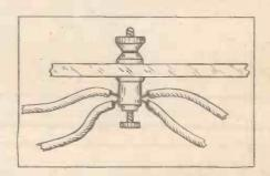
the accompanying sketch is to be recommended. A medium-size telephone terminal is fitted to the panel in an inverted position, and the hexagon nuts are replaced with two milled nuts taken from an ordinary terminal. Thus all soldering troubles are eliminated, the ends of the connecting wires being clamped in the lower terminal in the usual way.
