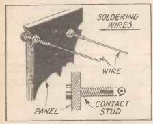
If it is preferred to keep heat away from the panel altogether, a short length, say two inches, of straight wire may be soldered to each screw or contact before assembly, making the screw, in effect, about two inches long. After assembly in the panel, the buswire is then soldered in the ordinary way to the end of this extension piece, the heated joint being now two inches from the panel.
