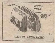
to the jaws of the vice. Then make the slot carefully by means of a hack-saw or a small tube-cutting saw. The barrel should be so placed in the vice that the screws (if they were in position) would be horizontal, the slot being then cut on the uppermost surface.
