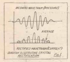
tions in the aerial, which try to force a current through the crystal alternately in opposite directions. But the crystal will only pass current in one direction, and therefore only those impulses which are in this direction will eause current to flow. The result is that, instead of very rapid alternations to which the telephones could not respond, we get pulsations all in one direction, whose varying amplitude gives an average effect of a frequency to which the telephones can respond."
