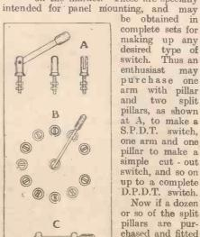
Now if a dozen or so of the split pillars are purchased and fitted to the panel in radial formation as shown at B, one has a very neat and efficient multiple switch.
