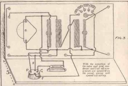
The back of the detector panel. The top connection to the variable condenser should be taken to the centre spindle instead of as shown.
