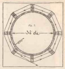
up to 480 metres the coil will require between 60 and 75 turns of wire.
