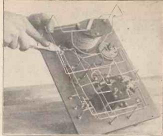
Fig. 5. A view of the lay-out and wiring at the back of the panel.
