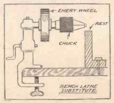
The emery wheel is in itself most useful, as it saves a lot of filing and sharpens drills, chisels and other small tools very quickly. Once the tool is fitted up there are all sorts of "small lathe" possibilities opened up to the ingenious amateur.
