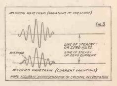
values of the fluctuations in the positive and negative directions respectively, and consequent value of the average "audio-frequency" current pulsations, depends on the sharpness of the bend in the curve. This may vary at different points in the same crystal, the curve when the cat's. whisker is resting on some points being practically straight (insensitive spot), and at others very decidedly bent (sensitive
