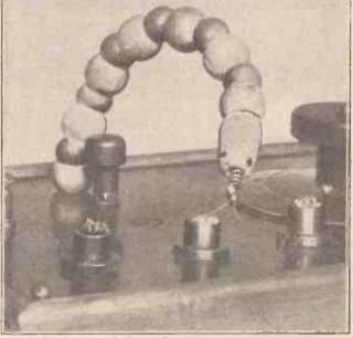
Fig. 6. One of the " fangs" making contact with the crystal.
