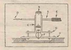
Note the whisker D is cranked, thus enabling a further movement to be given by knob E. F is a ball screwed to bottom of bracket and clamped between the plates G and H, thus giving the whole device a universal movement.
