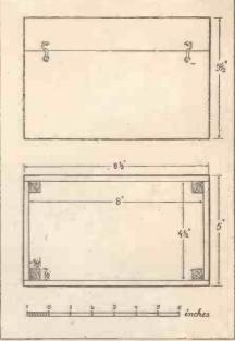
Fig. 9. The dimensions of the box.
