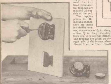
Showing how the switches are fitted. Fig. 4.
