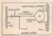
which winds up into a circular case by means of a spring. The case is mounted upon the wall at a convenient position, and an insulator with hook is attached to the end of the tape. A hook in the wall at another convenient place completes the device.
