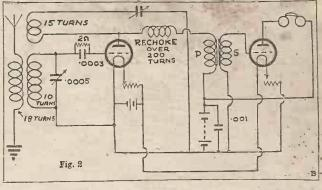
valve transformer is an ex-army one, 5 to 1 ratio.
