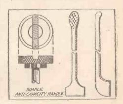
made any shape. Two are given here—one a spade type that will permit operation from above, the other to act lengthways. The spade pattern is filed out of a small strip of ebonits and milled or roughed at top for a grip; the bottom, of course, is filed to fit the groove in the knob. The other pattern is shaped as shown, but will not require to be milled.
