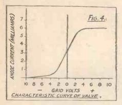
The steady anode current (which is always necessary with a valve) is supplied by the anode, or as it is commonly known, the H.T. battery.
