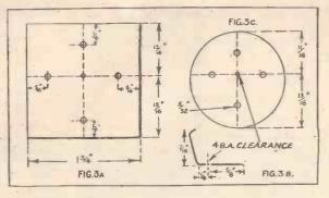
the brass contacts. The top plate is a circle of diameter  $1\frac{1}{2}$  in. cut from  $\frac{1}{8}$  in. thick ebonite, and four  $\frac{5}{32}$  in. holes are drilled in it as indicated in Fig. 3c.
