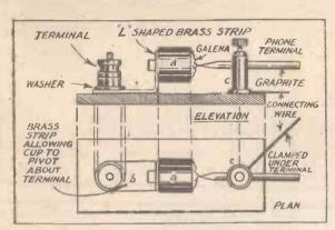
more permanent, has not the same sensitivity as Hertzite. Carborundum involves complication in the shape of a battery and potentiometer.
