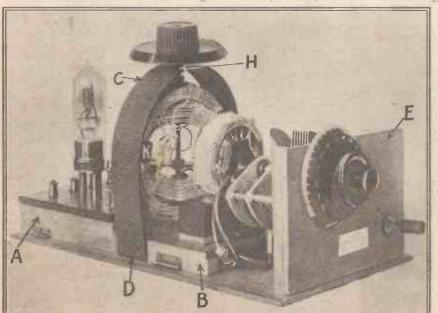
Fig. 3. The complete set. Note the position of the variometer in relation to the inductance coil.
