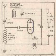
A simple single tuning circuit shorf-wave receiver which has been proved suitable for K D K A reception.
