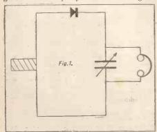
erative or straight circuit inductance. For use as wave-meter inductances these coils are particularly suitable, and if used for this purpose should be calibrated with a standard wave-meter and a graph made to show the different wave-lengths; the circuit of one is shown in Fig. 1.
