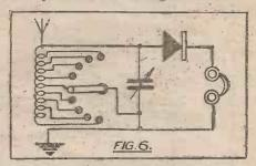
tapped coil and switch panel are screwed in position. The vertical panel with connecting wires to the crystal detector is next The front panel is the last to be atfixed. tached.
