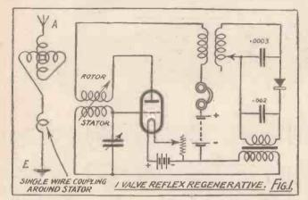
L.F., and infinitely purer owing to employment of crystal rectification, and its extreme selectivity enables one to tune out the local broadcasting stations, a thing utterly impossible with the majority of one or two valve circuits (Figs. 1 and 2).
