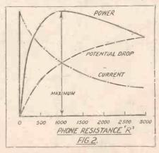
the circuit in which the telephones are inserted has an impedance in the neighbourhood of 10,000 to 20,000 ohms, and the impedance of the telephones should, therefore, approach as near as possible to this figure. In practice the telephone impedance seldom exceeds 5,000 ohms, but this is due to practical limitations due to the size of the telephone earpieces.
