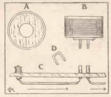
centre as shown at A. Over this hole is fitted a small piece of sheet ebonite, to which is attached two ordinary valve pins. The ends of the coil windings are connected to the nuts of the valve pins, inside the former.
