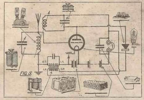
variable condenser to the right, when the panel is turned upside down for wiring. A short connection is taken from the aerial connecting wire to the grid of the valve. From both these wires two flexible leads about 12 in. long are soldered for connection to the fixed coil of the two-coil holder, which, as illustrated, is screwed to the inside left side of the case. The aerial circuit is thus completed.
