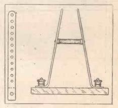
the left, and bent at the dotted line, so that when clamped to the ebonite base by means of the two terminals the distance between them is diminished towards the top, as shown in the illustration representing a view of the completed instrument.
