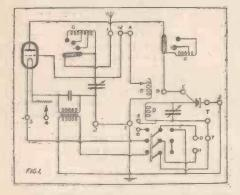
since its single valve is made to amplify the incoming oscillations before the crystal rectifies them, and also to amplify the rectified signals.
