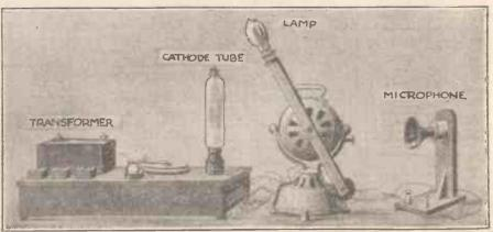
Figs. 1 and 2 show in the central pictures the positions of the mouth in pronouncing "o" and "e" respectively, the surrounding circles of lights being the actual flame pictures of the corresponding vowels. Above is seen Dr. Jacobsohn's apparatus for converting sound into flame fluctuations.
