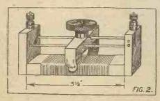
These are best made of  $\frac{1}{2}$ -inch ebonite, though  $\frac{3}{8}$ -inch or even  $\frac{1}{4}$ -inch material will do quite well. They are  $1\frac{3}{4}$  inches in height and  $1\frac{1}{2}$  inches in width. The drawing shows how they are drilled.
