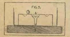
The metal case and carbon block can now be fitted to the wooden stand, as in Fig. 5. A large felt washer must now be fitted round the outside of the carbon, and this should be a trifle thicker than the block, so that when the diaphragm is fitted, as shown in Fig. 6, there will be a small space between it and the block.
