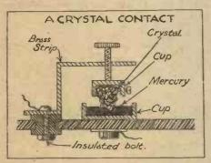
larger than the upper one, the latter being simply an ordinary crystal-cup inverted. A piece of springy-brass strip, bent twice at right angles, serves as a support for the upper cup, which is adjusted by the screw in the manner shown. 'The crystal should only dip just below the surface of the mercury. The crystal and mercury should, of course, be perfectly clean.
