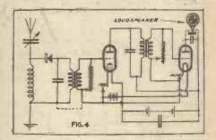
be used. The transformers should be placed well apart, and should be at right angles to each other.
