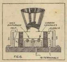
block should now be filled with small carbon granules, and the diaphragm then placed in position so that its coated side is next to the granules.
