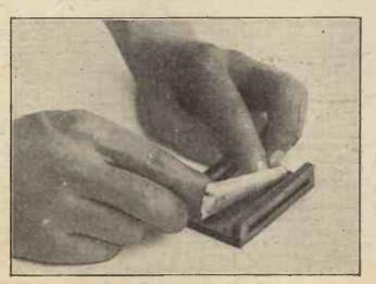
Fig. 2. Fixing the copper foil to the base.
