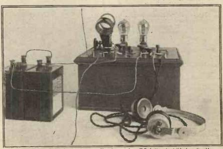
Fig. 2. The complete set ready for use. The absence of an H.T. battery is strikingly noticeable.
