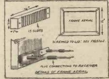
Fig. 5. Details of the frame aerial.
