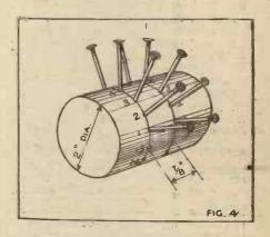
(the 70-turn coil, for example, will have exactly five layers of wire). The coil is then shellac-varnished and baked in the usual way while still on the former.
