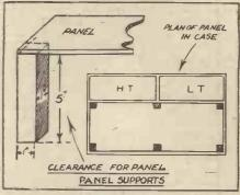
Fig. 4. The plan of the case and battery spaces.
