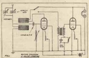
making up a simple two-valve set. The circuit diagram for this set is given in Fig. 1, and was published in POPULAR WIRELESS of June 21st, 1924.
