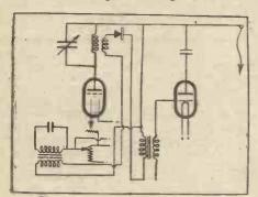
Fig. 2. Using a crystal detector instead of a valve.
