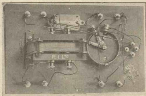
This photograph clearly shows the wiring. Note the pencilled leak across the Condenser.
