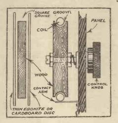
spring washers being included for proper fitting in the panel. The resistance coil is made from Eureka wire (about 20-gauge will be found suitable for general purposes).
