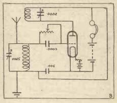
November 10th. The coils may be wound in basket fashion on  $1\frac{1}{2}$  in centre diameter formers. The aerial coil should have about 35 turns of 24 S.W.G. and the anode coil about 95 turns of 36 S.W.G.
