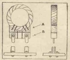
they are comparatively important wireless components, serving as plug-in mounts for home-made honeycomb coils.
