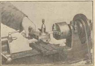
Fig. 24. Turning the ebonite knobs for the connector plugs.
