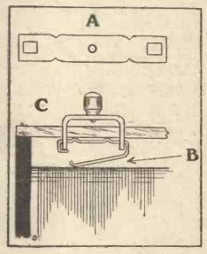
brass about 3/2 in. in thickness by 2 in. long is cut out as shown at A and provided with a rectangular hole at each end and a small screw-hole in the centre.
