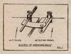
brass (a slotted keyhole plate) held in the input terminal of the next valve. This terminal is usually of the pillar type, and if not, a pillar type terminal can be readily substituted.
