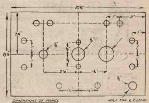
Fig. 3. Dimensions of the panel.
