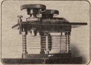
Fig. 6. The variable condenser with micrometer adjustment.
