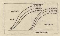
entirely disconnected, it gets more and more negative, and automatically shuts, only letting a few bold spirits rush the barriers. The finer the grid—i.e. the closer together the turnstiles, the easier does it shut.
