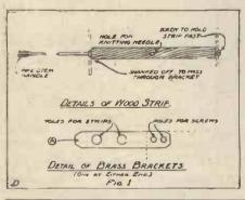
The tuner consists of three small strips of ebonite or wood—the writer used meat-skewers with pieces of a disused pipe-stem as knobs—about § in. square, the length being governed by the width of the tuner plus desired length of the extension handles. It is desirable to keep the outer one longer than the inner one to facilitate manipulation, and it should be at least 4 in. longer than the tuner to minimise body capacity effects.
