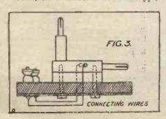
Fig. 1. After removing the contact screws (B) of one of the mounts, it will be found quite an easy matter to remove the plug and socket. Take one of the mounts and drill a hole at C to take the brass plug and tap a smaller one to take the contact screw on the rear end. After inserting the plug screw the contact screw well home to make the plug secure, Fig. 2 (a). The other mount should now be similarly treated and the brass socket secured, Fig. 2 (b).
