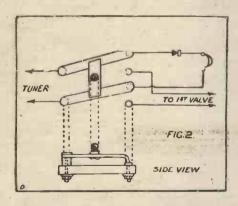
then simply push over the switch and light the filaments. Of course, this type cannot always be used as, in the act of changing over, the switch arms each touch two contacts instead of one, finding sometimes a new path for the H.T. current with disastrous results. In this case an obvious remedy is the provision of two extra "dead" studs in addition to the four studs in use.
