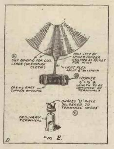
The coil pivots are made from  $2\frac{1}{2}$  in. lengths of 8 in. ebonite knitting needles, pointed each end and one end screwed into the centre of each strip at the point indicated (see Fig. 1). These rods are supported by brass brackets  $1\frac{1}{2}$  in. by  $1\frac{1}{2}$  in. by  $1\frac{1}{2}$  in. thick, holed to receive the strips and screws for fixing at A, Fig. 1.
