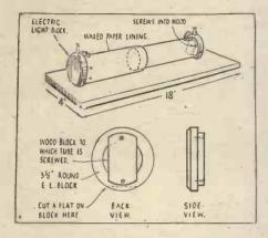
few pence and a little patience. The following instructions are for the construction of a cheap condenser, and by little additions, according to the amateur's fancy, it may be made quite a smart-looking instrument.
