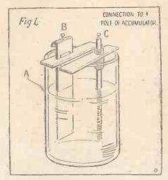
a piece of wood which rests on the top of the jar. The aluminium is made fast by passing it through a cork, and the iron is wedged it in, as shown in Fig. 1. At the top of each electrode is a screw for connecting wires.
