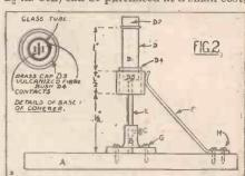
and the movement consisting of an electromagnet with armature, also hammer, should be removed from the bell-base board, and suitably mounted upon the wooden base A (Fig. 2) in such a manner that when the electric bell movement in question caused to function its hammer should strike the brass cap D3 fitted to the coherer
