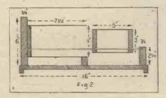
to the full depth that the screws will take; otherwise, owing to the hardness of this particular wood, difficulty would be experienced in driving them right home. A few turns with a large drill should be made to countersink the heads of the screws to the surface of the wood.
