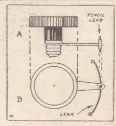
The pencil lead should make just sufficient contact with the leak to ensure a good connection, and should not be pressed tightly on to the leak, for obvious reasons.
