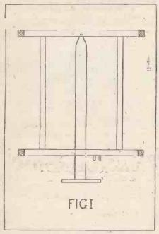
A frame aerial is also frequently referred to as a "closed" or "loop" aerial, and of these terms the latter best expresses its particular character. That is to say, an ordinary loop of wire constitutes a simple direction-finding aerial.
