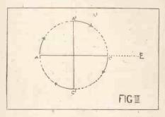
This merely means that, with reference to any particular transmitting station, there are two maximum and two minimum positions for each frame aerial. Reference to Figs. 2 and 3 will make this clear. Fig. 2 shows the plane of a single loop aerial. The line with the arrows, drawn across the plane, shows the two directions from which maximum signals could be received. Similarly, if we imagine the transmitting station at E, maximum signals will be received whether the side AB or CD is nearest to it.
