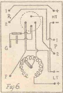
left-hand side of the case by means of a piece of fibre screwed across it to clamp it, or by four screws, so as to come just under the terminal G when the panel is placed in position.
