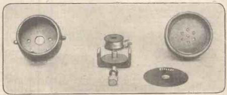
Component Parts of the Watch Receiver Telephone.
