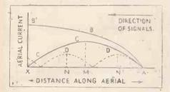
in shunt or in series. The purpose of adding these electrical elements is to control the velocity with which the current wave induced by the received signals travels along the aerial.
