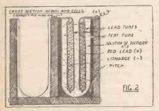
then filled with red lead and the other with litharge, the open ends being squeezed for  $\frac{1}{2}$  in. to close them up. The positive tube will be the one filled with red lead (oxide of lead); 16 tubes with red lead and 16 with litharge will be required.
