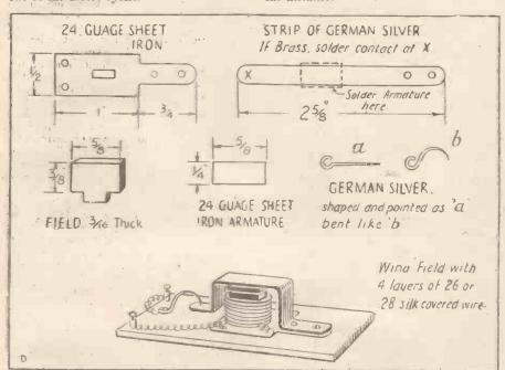
Making a Small Testing Buzzer.
