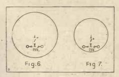
the wood and drill half-way through from the one side and complete the drilling from the other. To obtain exactly similar positions pins should be fixed to the centre and a thread with a small weight suspended from each side. If 1.18 in. radius circles have been drawn on both sides it will be a simple matter to mark the centres of the holes so that they will be exactly in line.
