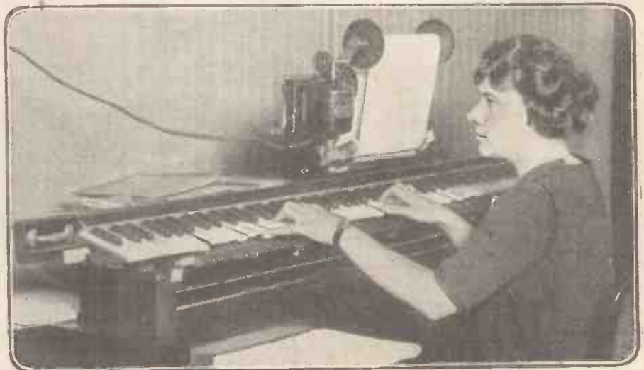
The musical typewriter—a new device for playing the piano by wireless.
