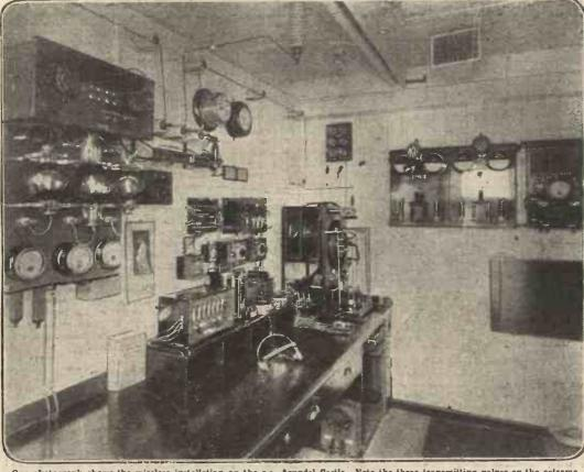
Our photograph shows the wireless installation on the s.s. Arundel Castle. Note the three transmitting valves on the extreme left, and just below them the seven-valve Marconi Amplifier, and the Type 31. Crystal Receiver. On the extreme right is the "spark" transmitter. A quenched gap is used. The "change over" switch for connecting one or another transmitter to the aerial is seen a little to the left of the first clock.
