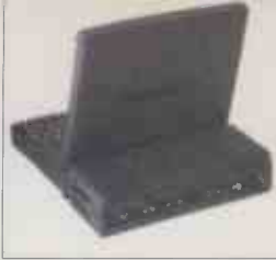
There are two docking stations available, the EZ Dock for the T5000 and the Dock Mate for the T5100 both offering greater connectivity
