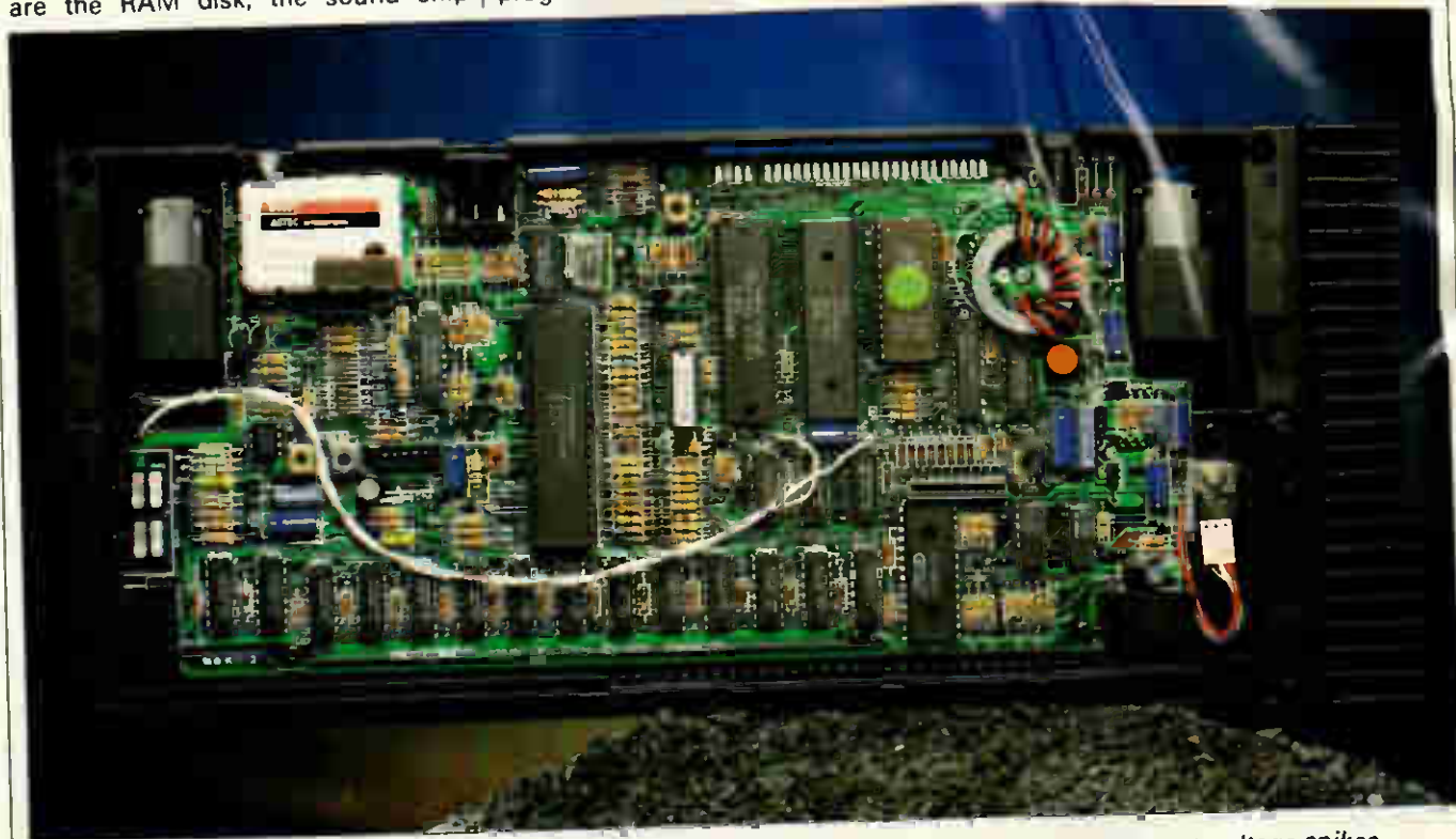
Inside: the new-format circuit board includes a sound chip, and lots of cheap diodes to prevent voltage spikes
