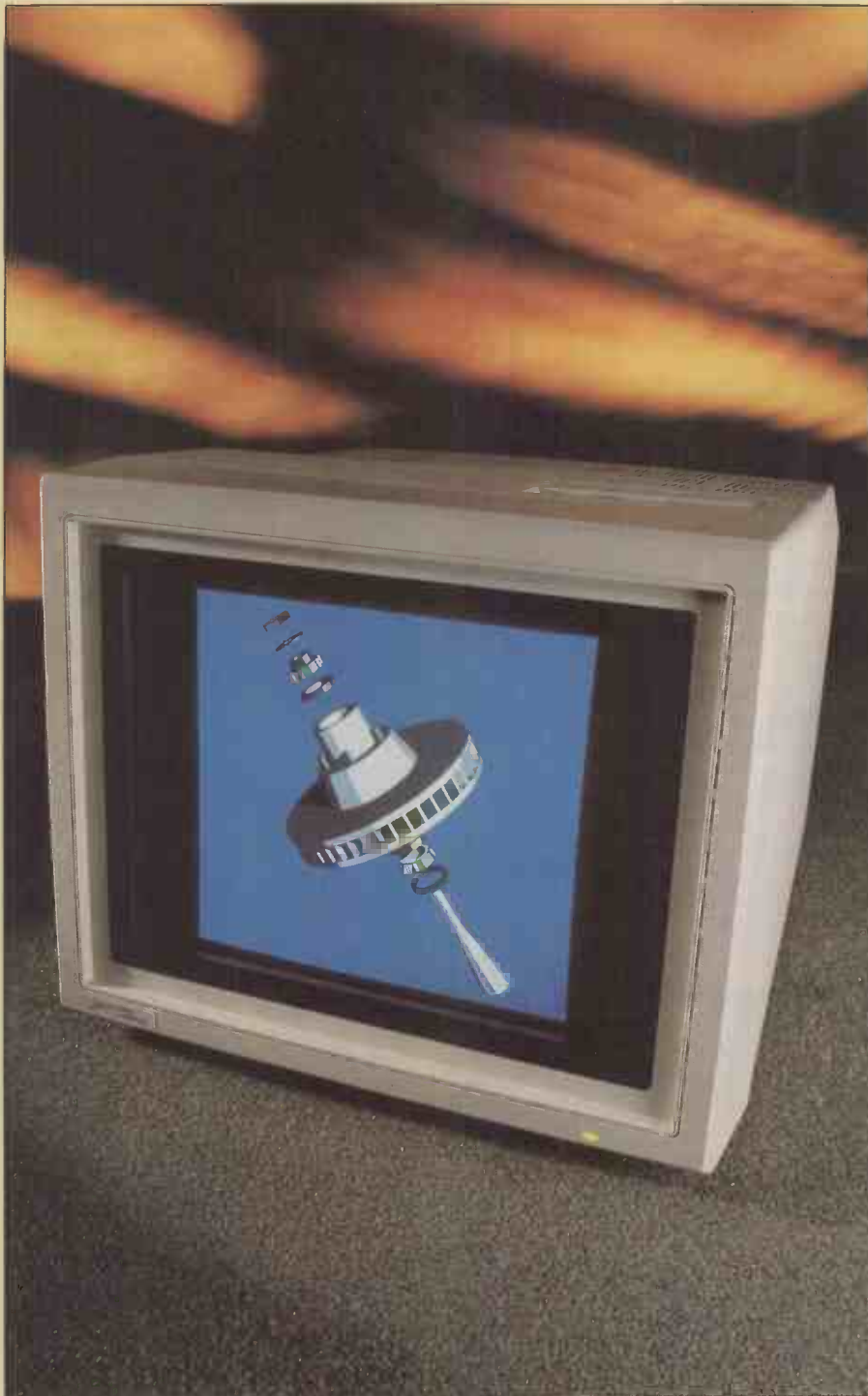
The Flat Tension Mask monitor is available on a range of Zenith machines. Exposure to conventional curved monitors means that, for the first few days of use, the screen appears to be curved inwards
