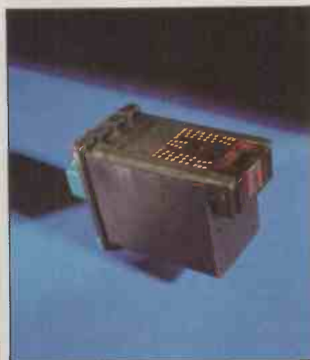
The removable print head also contains the ink reservoir. The large gold plate is the electrical contact, the small one underneath contains the ink nozzles.
