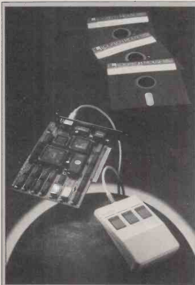
Usually, mice for the PC family are plugged into a dedicated mouse board, or into the keyboard, or into a serial port. Logitech has decided that most people will want the mouse when they upgrade to high-resolution graphics, and so has launched a combined EGA screen card plus mouse. Software with it includes a Microsoft Windows driver. And there's also a light pen interface.
