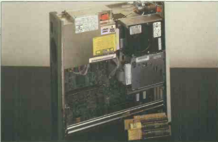
Surface-mount technology features largely on the 'Planar' or motherboard. The detachable expansion bus also houses the CMOS RAM back-up battery. The Inmos chip (bottom left) holds the colour look-up table
