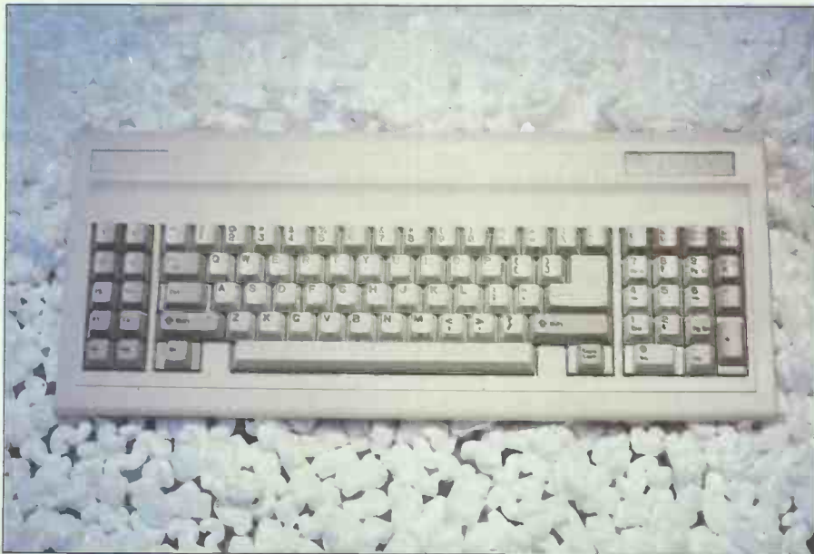
The AT-lookalike keyboard has a steel rather than a plastic base, and is also heavier than most clones; this reinforces the machine's 'solid' look
