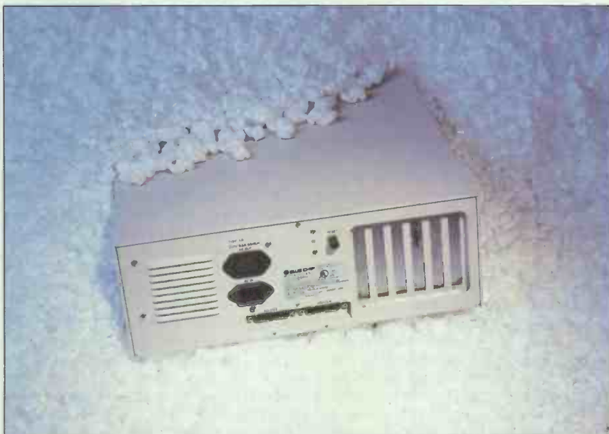
Unlike most PC clones, the Blue Chip only has six expansion slots
