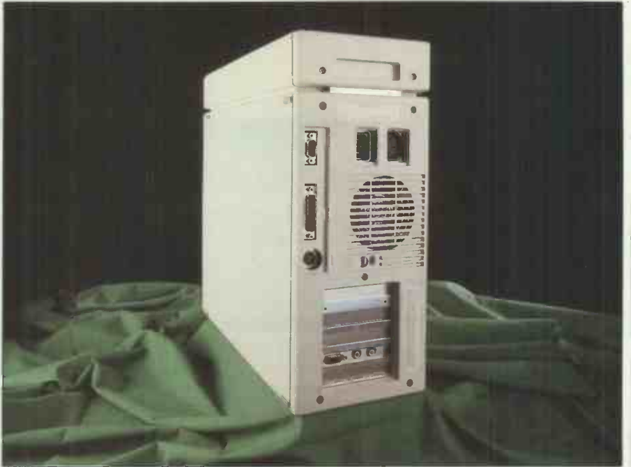
A standard selection of ports is present. The detachable floppy disk sits on top of the system box when it is vertical and looks like a silly hat
