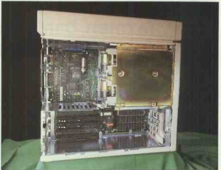
Inside the PAC286: the two battery-like objects in the centre are the stepper motors, one for each disk drive
