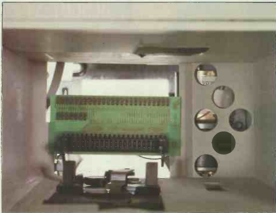
The mechanism which pulls the Data Pacs into the system is innovative but could give cause for concern
