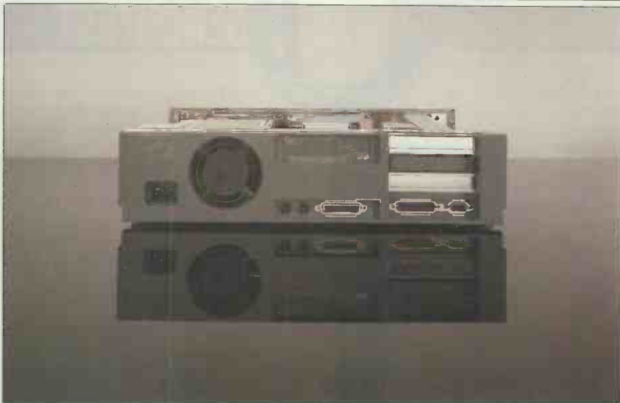
Apart from the non-standard keyboard and mouse ports, the rear of the Model 30 holds few surprises. The horizontal expansion slots are initially covered by grey plastic plates. The fan is almost silent
