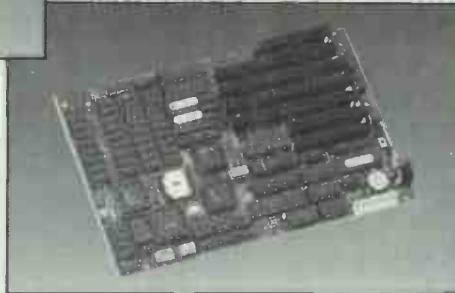
DIGIS-286S "Mini" AT High-speed Motherboard * 6/8 or 6/10MHz at 0/1 wait states. * 1 serial port on board. * Standard mounting holes for XT or AT case.
