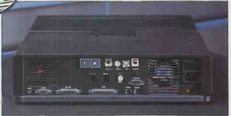
The rear of the Dynamac has been utilised to the limit. Most ports have been inherited from the Mac Plus, with additional slots for an internal modem and networking facilities.
