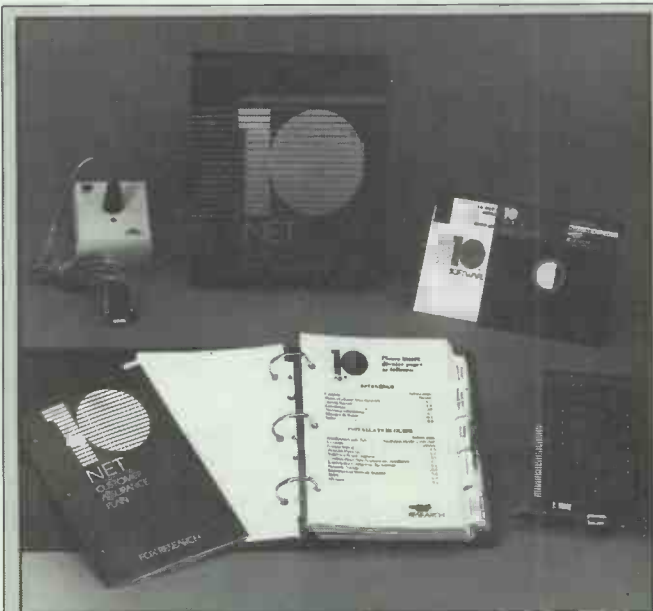
The local area network supported by Olivetti in this country is the Fox Research 10-Net. These boxes are the methods offered by Fox to attach fibre-optics to a 10-Net installation. Eventually, that will mean enormous improvements in speed and security for network users.
