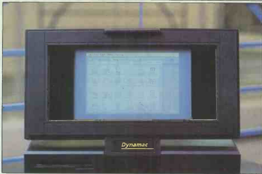
At 640x400 pixels, the Dynamac's power-hungry electroluminescent screen is 46 per cent bigger than the standard Macintosh unit
