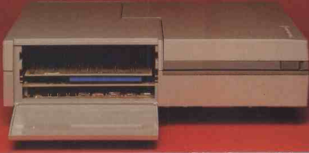
Two of TI's forthcoming range of option modules can be placed in these spaces
