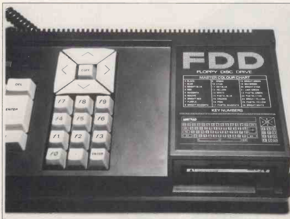
The bulging right-hand side now includes an integral 3in disk drive
