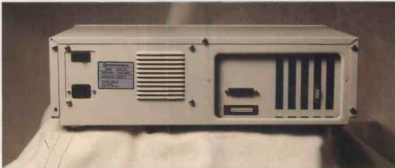
The back panel is constructed of metal and incorporates only the bare minimum of ports
