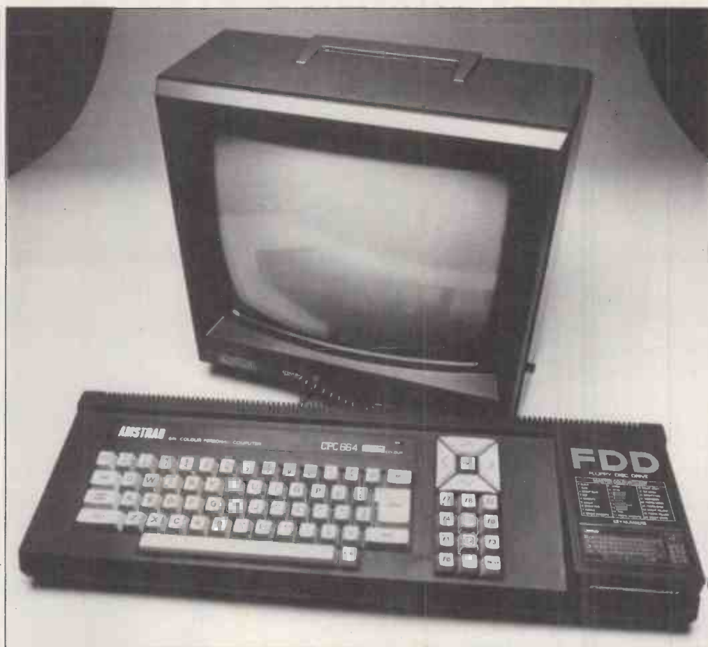
The CPC 664 incorporates the CPC 464 with Amstrad's disk drive in one unit
