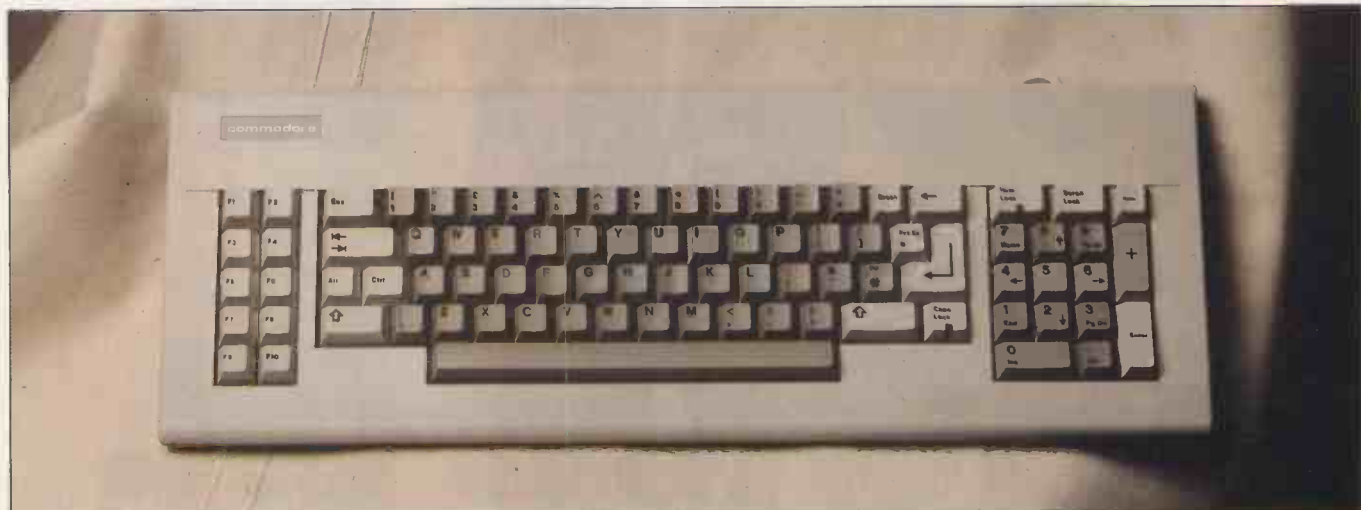
The Commodore PC's lightweight keyboard is similar in style to that of the IBM PC, but with some detail changes
