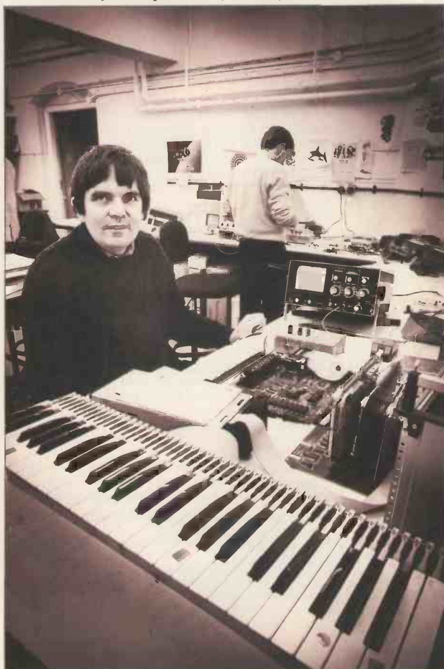
A prototype music synthesiser, an EPROM burner & one of Notting Dale's staff.
