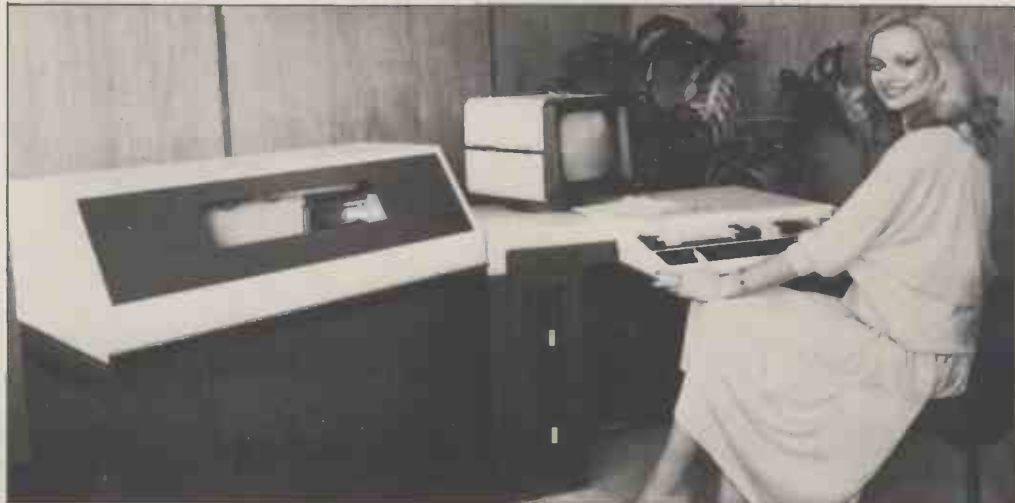
At £8500 with an enclosed (quieter) printer, two floppy discs and screen/keyboard, this Triumph Adler 1100C is a big change for the company. It was launched at the IMEC exhibition and the maker claims it is on one-week delivery from order.
