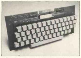
The versatile interface allows user selection of parity, positive or negative logic data and strobe outputs, alpha lock operation and both D.C. level and pulse strobe signals. A latching shift lock key is included, and all outputs are TTL-DTL-MOS compatible. The KB756 is economically priced at £60,00, and discounts
