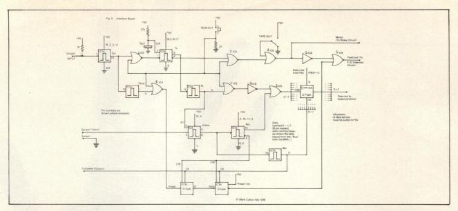
The interface handles all the timing and logic, but the TTL output levels it produces do not supply enough current to activate the solenoids, so a Darlington pair (Fig 4) amplifies the current to activate the solenoids whenever instantaneously required.
