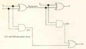
In Table 2 the partial carry (1) is formed by the logic And operation (X AND Y). The first half adder forms the partial sum by the operation X exclusive OR Y.
