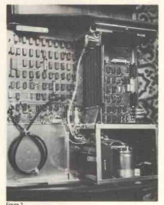
Figure 2. Main PCB, backplane and power supply fitted into chassis.
