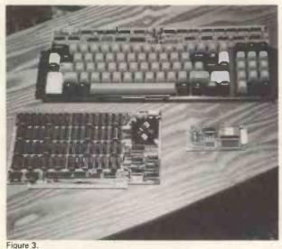
Keyboard assembly, 8K static RAM memory board and 'SOLOS' personality module
