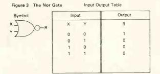
owners of the car park want to know if they are making a profit (car park full), a loss (car park empty) or breaking even (one car in the park). Obviously the AND gate can detect a profitable state and the NOR gate a loss. The exclusive OR can be used to unambiguously detect the state of breaking even. Notice here that the inclusive OR could not distinguish between profit and breaking even.
