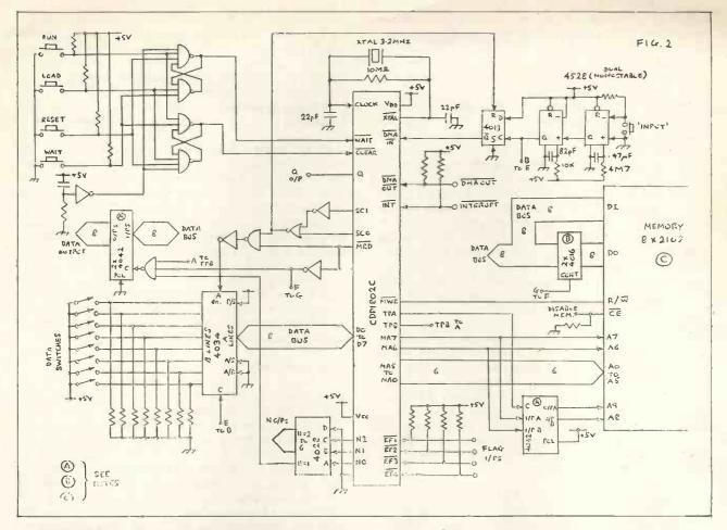
The D.M.A. facility is worthy of special mention, since it allows the easy entry of programs and data without special ROM's or extra external logic to gain direct access to the memory system. It is this D.M.A. facility that makes the 1802 particularly attractive to people new to M.P.U's.
