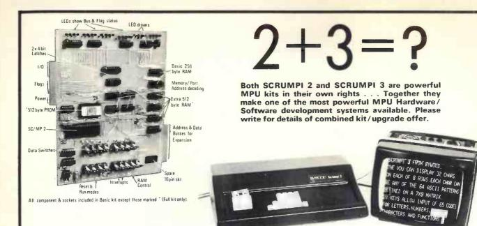
SCRUMPI 2 is a single board MPU system based on the SC/MP2 microprocessor chip. Switches allow Single-step/Halt/Run modes with PROM or RAM bootstraps. RAM protect and interruption. Basic kit includes all IC sockets, all ancilliary components, SC/MP2, drivers, decoders, latches and 256 bytes of RAM. Full kit includes additional 512 byte PROM & 512 byte RAM.
