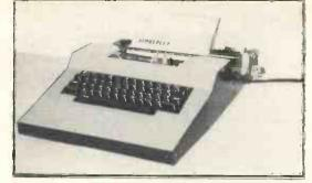
Designed for parallel data input with handshake control. ASCII coding is accepted for the 88 characters available, operating at a speed of 8 cps from a standard peripheral interface. It is supplied fully built and cased at £200 (including carriage and VAT). Alternatively, as a print mechanism only, requiring all power other than 240V, case, and TTL logic to be added, the cost is £160.
