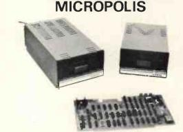
Micropolis disk drives employ higher standards of engineering to pack either 143K or 315K bytes per diskette, formatted, Supplied complete with controller card, cables, manual and software they plug directly into the S100 bus; 8080 or 280.
