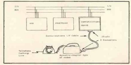
Fig. 1. Single-Line Communications Board
