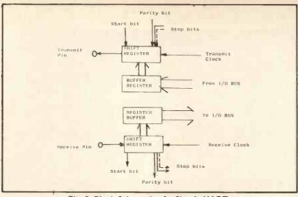
Fig. 2. Block Schematic of a Simple UART
