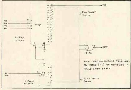
Fig. 1. Address Bus Decode
