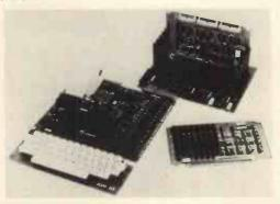
The AIM 65 expansion motherboard have five connector slots that can accommodate any of the Rockwell System 65 modules or Motorola Exorcisor modules, as well as add-on modules from Burr-Brown and other manufacturers.
