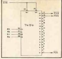
Fig. 4. Peripheral Decode
