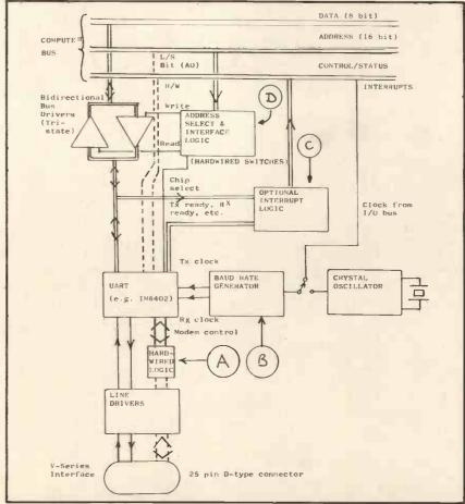
Fig. 3. General Schematic of a Communications Interface Board
