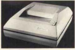
RS232C Serial Interface is supplied as standard with parallel and current loop interfaces being available as options. Baud rate is switchable up to 9600 baud and the Print Head is microprocessor controlled with a full 2 line buffer and 96 character overflow. (No price quoted to PCW).
