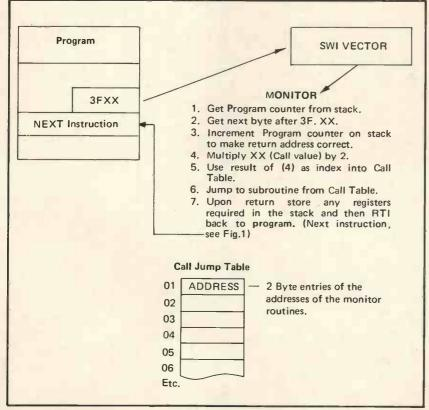
Fig. 1. Call Mechanism
