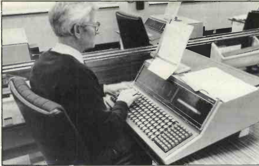
An operator working at an input keyboard. Under the Mirror Group Newspapers system, all text is normally keyed directly into the computer via input keyboards. These replace the functions of both the linotype and Ludlow operators. Photo: Daily Mirror
