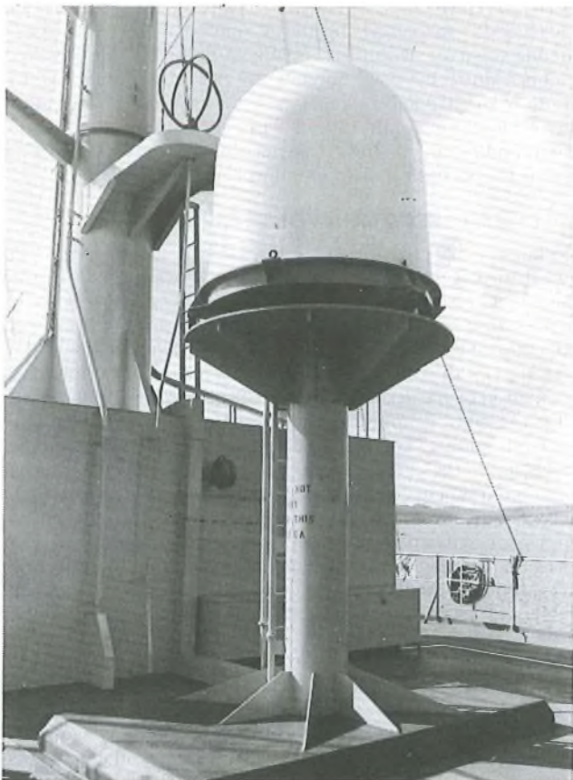
FIG. 5—Typical antenna installation showing radome weather protection (Photograph by courtesy of The Marconi Company Ltd.)
