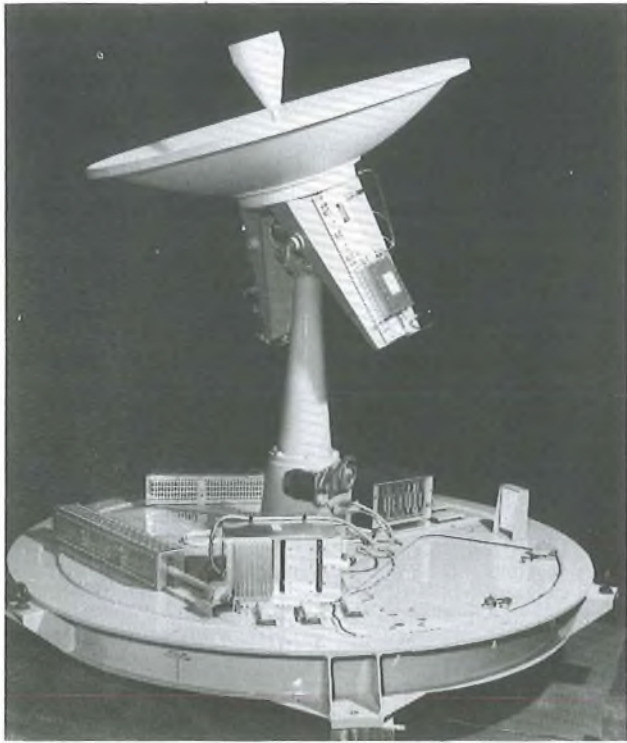
FIG. 4—1.2 m antenna and low-noise receiver (Photograph by courtesy of The Marconi Company Ltd.)
