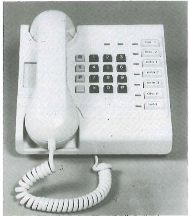
Note: Labels indicate instrument is extension 4 of a 2 + 4 system
