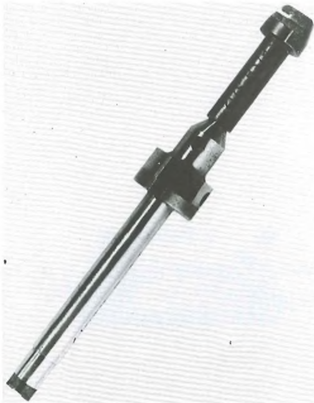
FIG. 3—Wire-wrap head in cutter/holder
