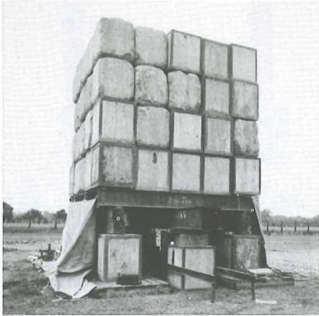
FIG. 10—Kentledge system of pile testing
